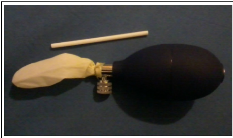
Fully Constructed (dental floss wrapped 20-30x around finger cot. Toothpick/Q-tip with snipped ends)
