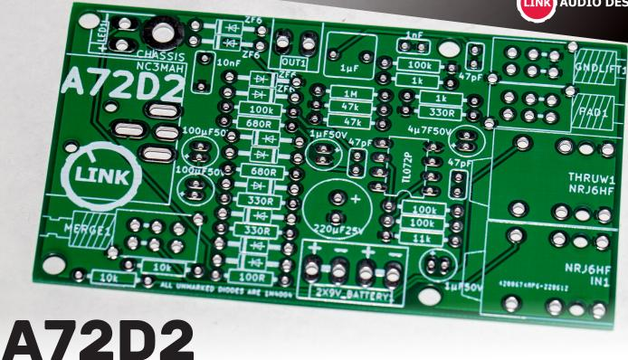
Let me Introduce this nice Direct Injection Box as Active Version. I have designed this DIs in Business Card Format 85x55mm. This Version work with different Consoles or Preamps. This Version has Ground Lift, Pad and Merge Function. For the Active Version you need a Battery Supply or 48V Phantom Power from the dedicated Preamp. It's basically inspired by LA AUDIO Active DI Box.
