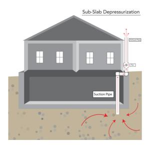
The EPA approximates that a radon elimination system sets you back regarding \$1,200 for an ordinary house. The system is generally comprised of one or more PVC pipes that run from the radon-emitting dirt under a house up with the roofing system. An in-line fan draws air via the system to make sure that it does not leach into living rooms.
