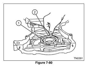
Using a feeler gauge, measure the clearance between outer rotor (1) and the oil pump case rotor bore (2). If the clearance is beyond the service limit, replace the oil pump assembly.
