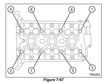
5. Tighten cap screws (1 through 8) in sequence, to specification.
