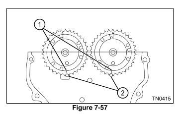
2. Apply engine oil to camshaft journals, lobes, and timing sprockets. Align timing gear dots (1) with the index marks (2) on the cylinder head.
