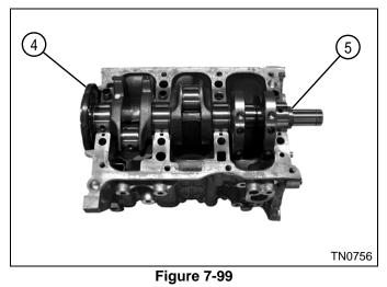
8. Remove rear main seal (4) and crankshaft (5).
