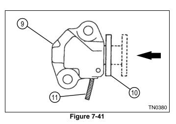
Release tension adjuster (9) manual lock using a rod 5. (11) approximately 0.8 in. (2 mm) in diameter. Depress the lock with the rod and reset the piston (10) as shown.
