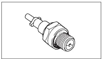
Figure 8-6: Compression Gauge Hose Attachment B
