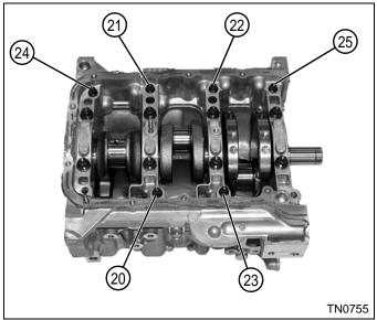
Figure 7-106: Torque Sequence M8 Cap Screws
