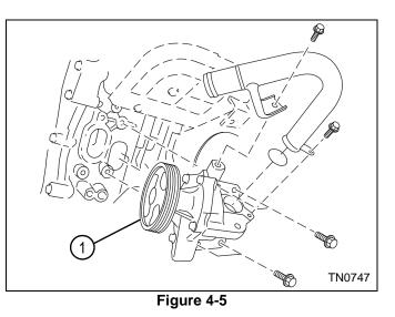
The engine is equipped with a belt-driven water pump (1) driven from the crankshaft pulley. The water pump circulates coolant throughout the entire cooling system. The water pump is equipped with a "weep hole" for indication of seal wear. The pump is serviceable as a unit only.
