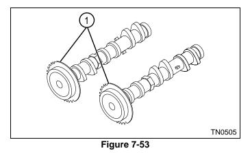
Inspect the camshaft timing sprockets (1) for wear and damage. If any abnormal condition is noted, replace the sprocket.
