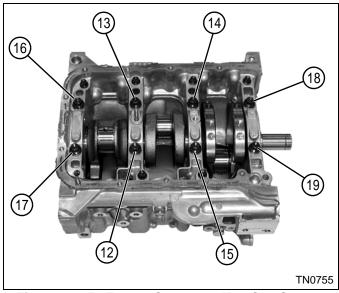
Figure 7-105: Torque Sequence M10 Cap Screws
