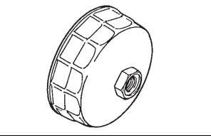
Figure 8-1: Oil Filter Wrench
