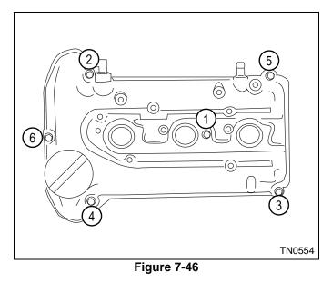
Tighten cap screws (1 through 6) in sequential order as shown. Torque cam cover cap screws at increments of 32 lb-in. (3.6 N•m), until specification is reached.
