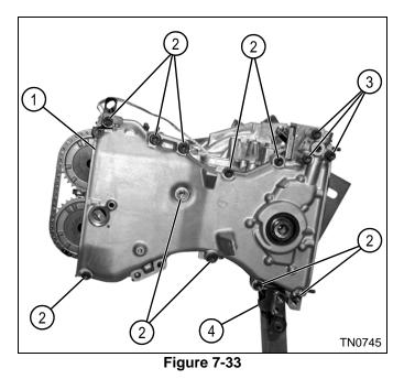
9. Remove idler pulley/alternator bracket (4).
