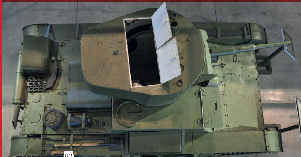
The T-26 M-1933 was a Soviet development of the 'Vickers 6 ton' tank, mounting the same turret and armament as the BT-5 and early BT-7 fast tanks
