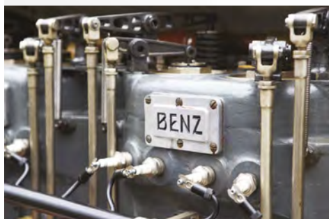
Dials are low on the driver's worry list. Below, naked rockers of twin-plug four, with blocks cast in pairs
