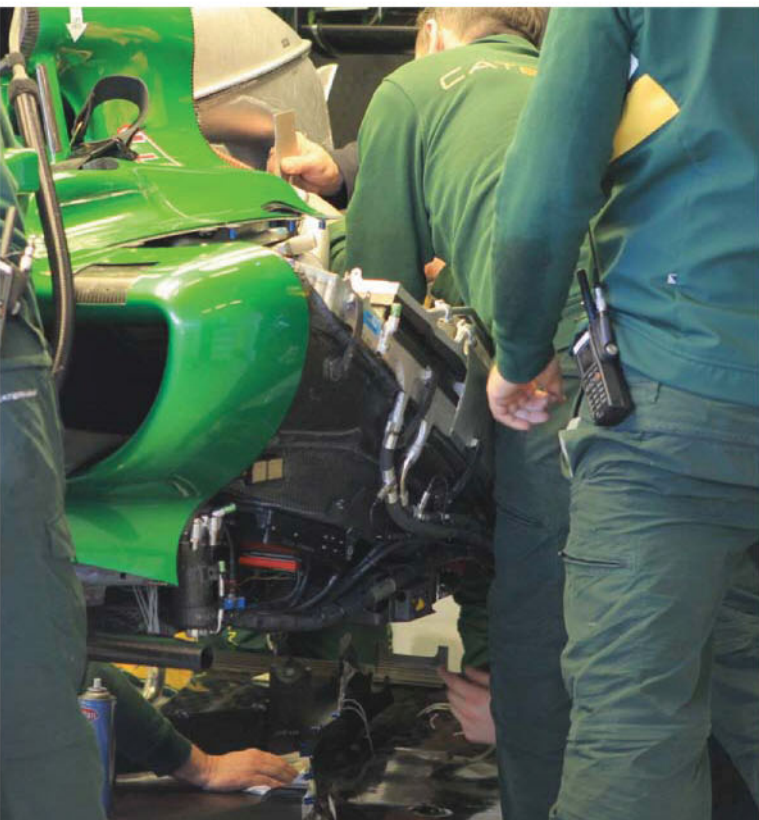
The cooling system on the cars is proving to be a major packaging issue. Here on the Caterham CT05, two heat exchangers are visible, as is the lower side impact structure
