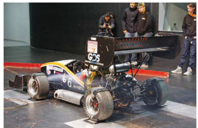
The left side featured the exhaust tailpipe and heat shield
