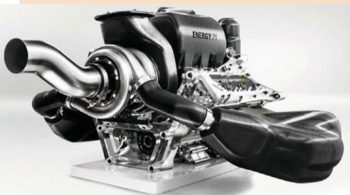
Renault's RS34 engine is fitted with a ballistic cover around the turbocharger when installed in a car, the Ferrari engine is not
