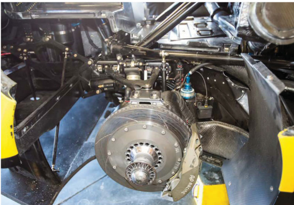
The C7R features a new cradle at the front and the rear for the engine and the gearbox. They are more robust
