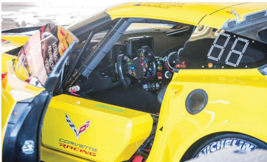
The C7R has a new side impact protection system, made from carbon Kevlar with an expanded honeycomb interior
