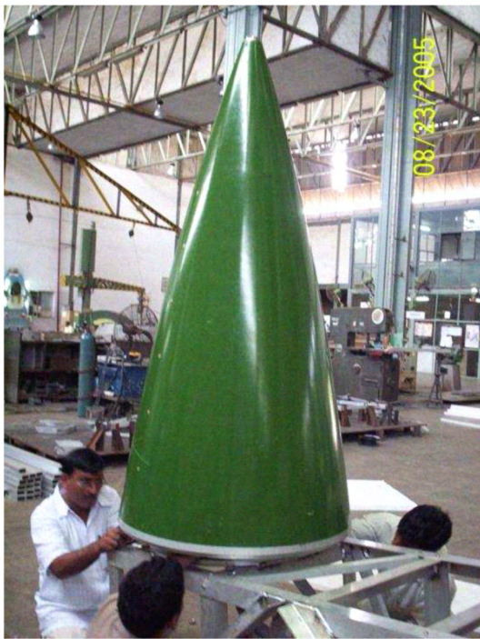
Figure 5 Radome on fixture
