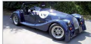
2008. Roadster Lightweight class B race car. Bare chassis rebuilt by us with great attention to weight saving to full class B specification in Aero Racing Morgan Challenge Race Series. Including 4 wheel disc brakes vented at the front, 7" x 16" Image wheels with 225/50VR16 Yokohama tyres, modified 3 litre Ford V6, with bespoke ECU, race cams, and big bore manifolds giving circa 280BHP at 7000RPM. She wants for nothing and is ready to race. £39,850
