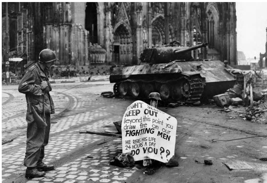
Days after the battle a corporal looks at a warning sign posted in front of the burned-out Panther. By now the turret has been rotated to get the gun barrel out of the way and the muzzle brake has been removed.
