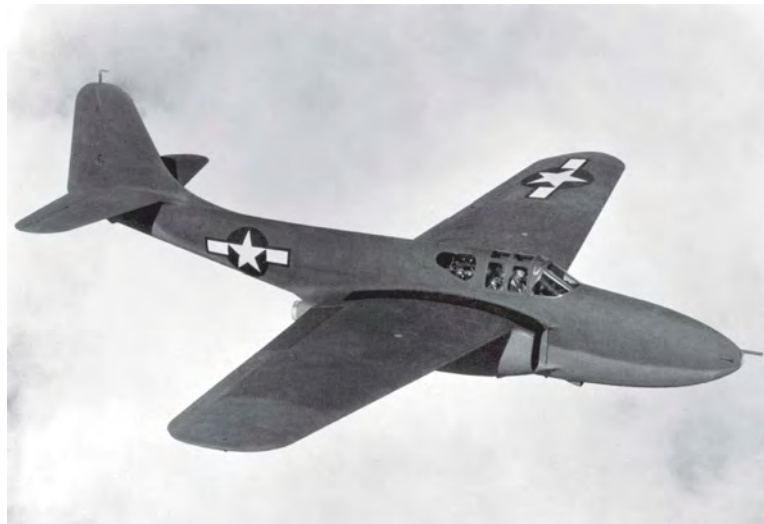
LEFT: A pre-production YP-59A, complete with nose armament, in flight.
