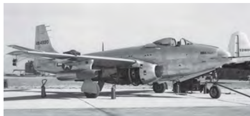
ABOVE LEFT TO RIGHT: A very rare image of the complete second prototype, 44-84991, with its extended nose and larger tailplane; and the first XP-83 is prepared for its ramjet flight trials, which only lasted one sortie before the aircraft was lost. One small Marquardt RJ30 ramjet, of just 21in (0.533m) diameter, was fitted beneath each wing. VIA GERALD BALZER
