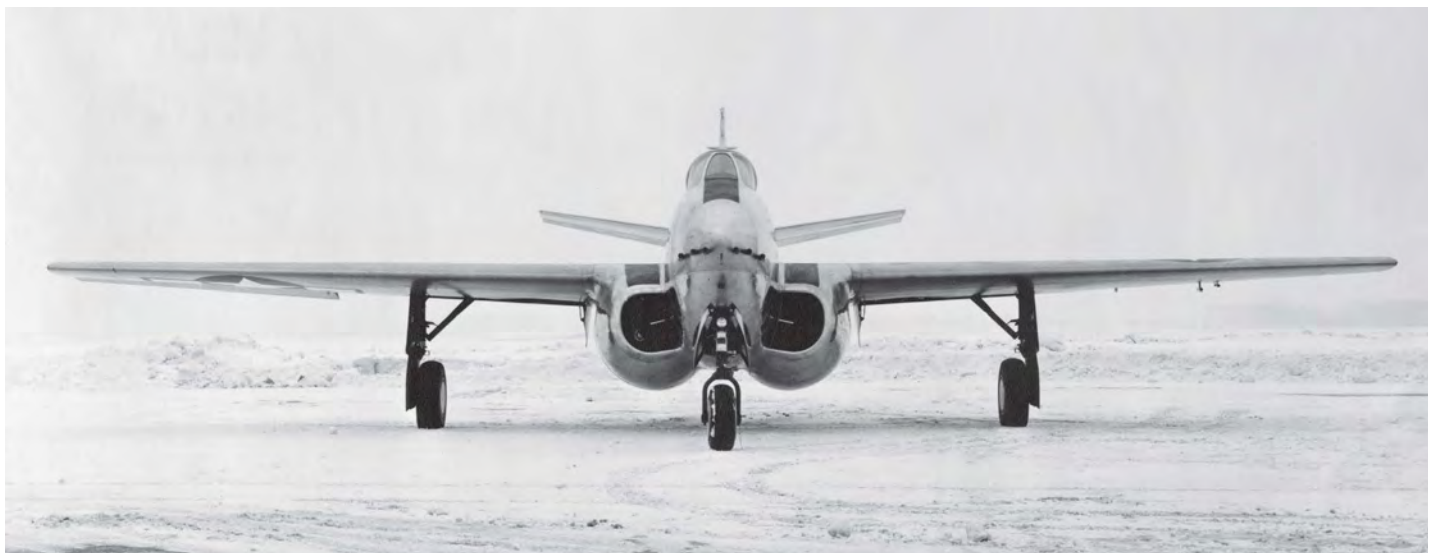
BELOW: One of a series of walk-round views taken on 8 February 1945, the day the XP-83 was rolled out, this head-on view shows the large air intakes and wide-track undercarriage. The fuselage itself was quite slim.
