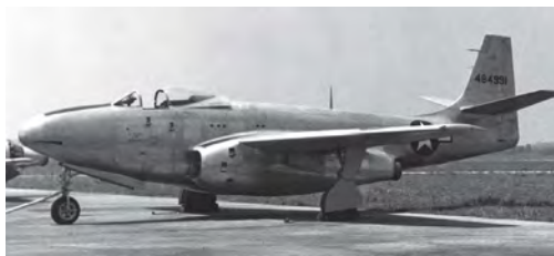
ABOVE LEFT TO RIGHT: A very rare image of the complete second prototype, 44-84991, with its extended nose and larger tailplane; and the first XP-83 is prepared for its ramjet flight trials, which only lasted one sortie before the aircraft was lost. One small Marquardt RJ30 ramjet, of just 21in (0.533m) diameter, was fitted beneath each wing. VIA GERALD BALZER
