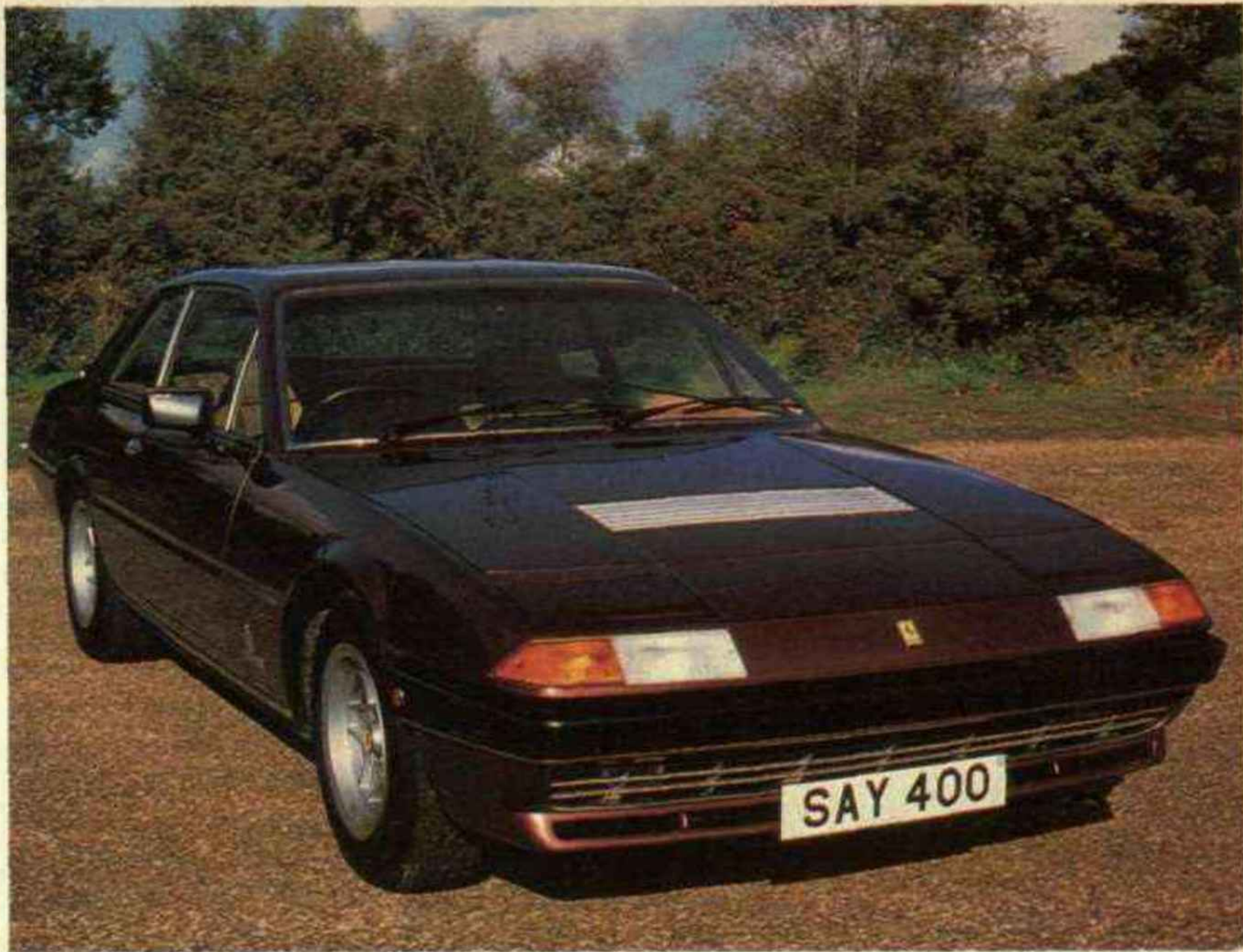
The Pininfarina body features retractable headlamps, daylight flash/fog lights inset in the low grille and a grille in the bonnet top.
