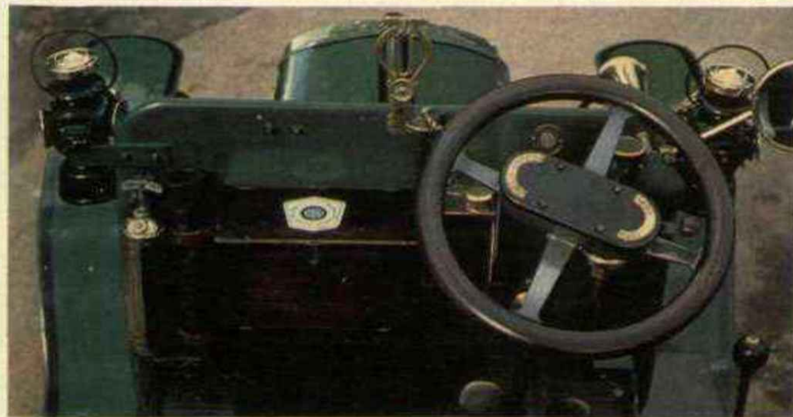
Thornycroft details:— Top left, as the driver sees it; note the unusual quadrant for the throttle and ignition levers; below, the platform rear springing. Right, off-side of the engine showing the long inlet tract that feeds automatic inlet valves on the n/s, and the small-bore of the water-pipes.
