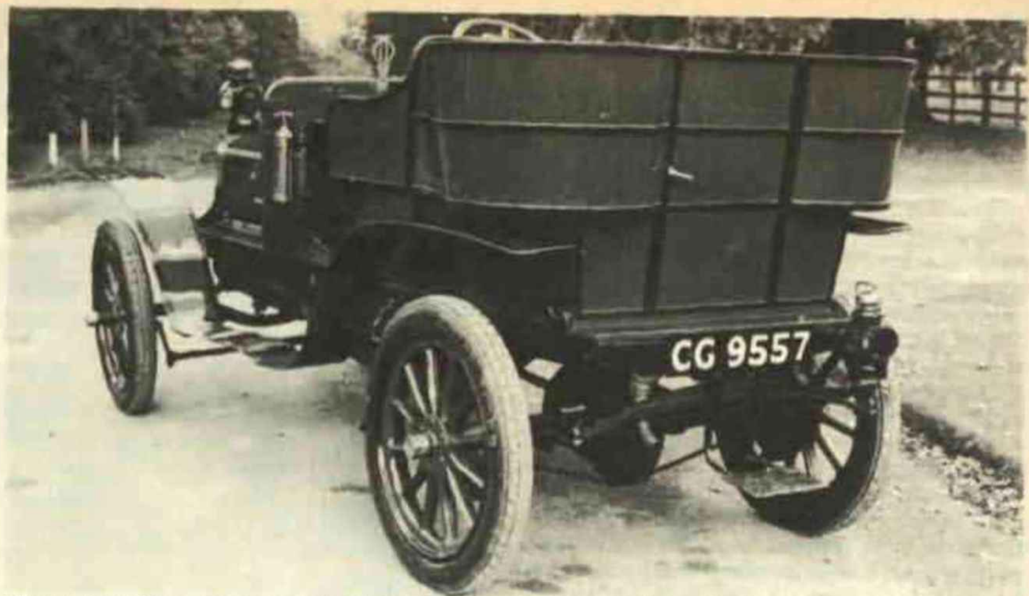
The big 1904 Thornycroft owned by BL has a rear-entrance tonneau body. Note the transverse platform spring which augments the rear half-elliptics.
