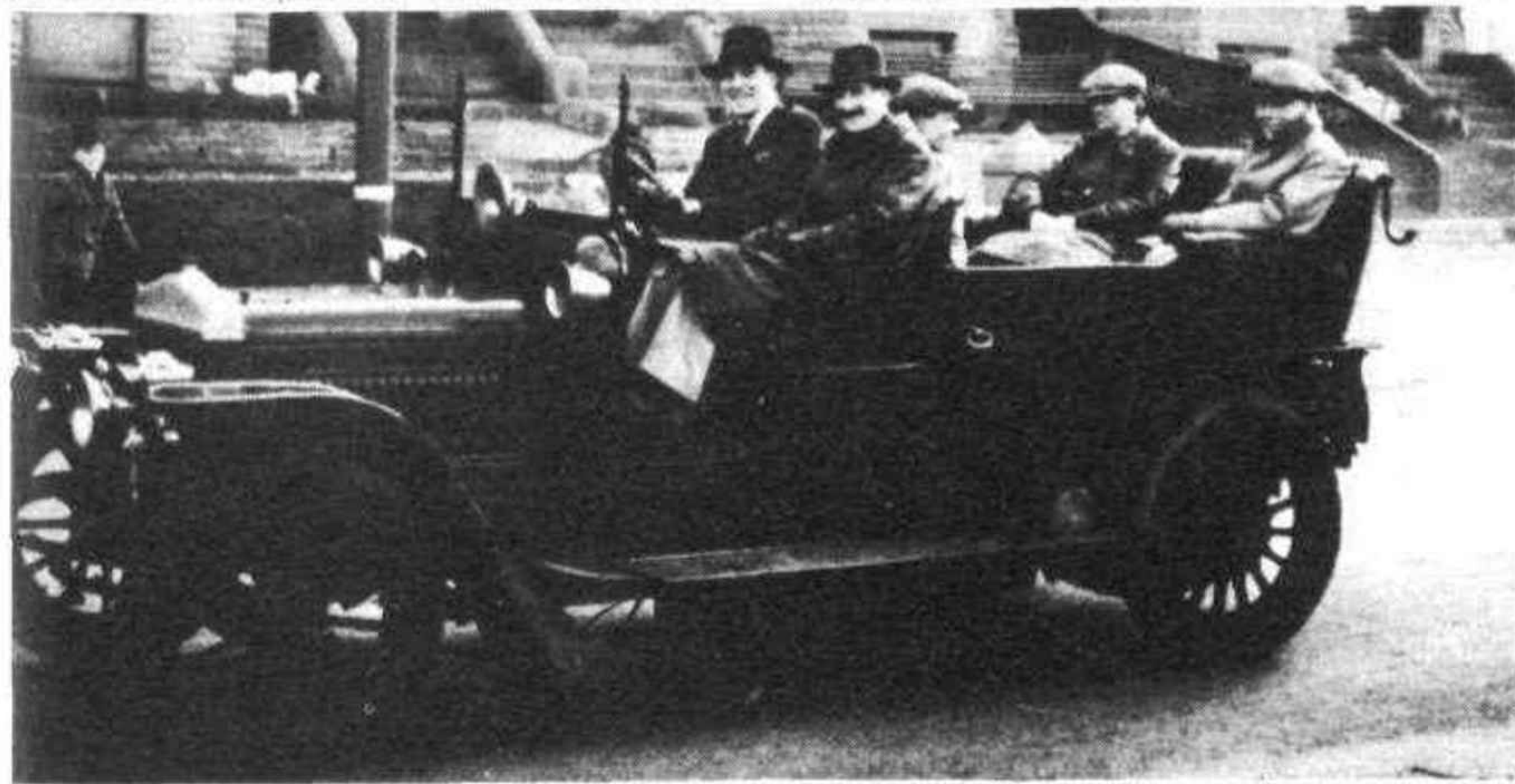
This Daimler, featured in MOTOR SPORT in April 1937, had a 9.2-litre double sleeve-valve engine, but from the specification its chassis could have been from an earlier poppet-valve car used during the experimental period with the Knight engine. Kent Karlake, the one-time old-car correspondent in MOTOR SPORT under the pseudonym "Baladeur", is in the front passenger seat, Cecil Clutton and Anthony Heal, well-known VSCC committee members, are in the rear and we think the driver is W. G. S. Wike.
