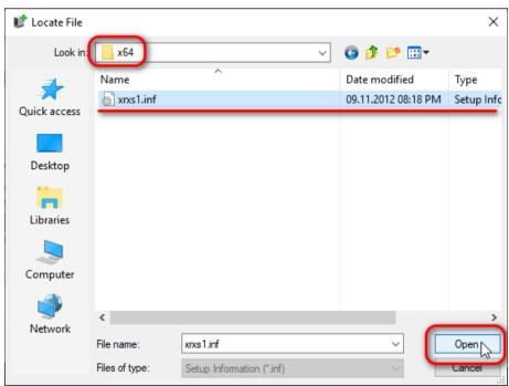
Depending on your operating system's architecture (32-bit or 64-bit), you need to load either the .inf file from the x86 directory (for 32-bit OSes), or from the x64 directory (for 64-bit OSes). In this particular case, I'm installing the driver on a 64-bit (x64) OS, so that's why I'm positioned in the **x64** directory. If I were installing this driver on a 32-bit OS, I'd be positioned and loading the **xrxs1.inf** file from the x86 directory.
