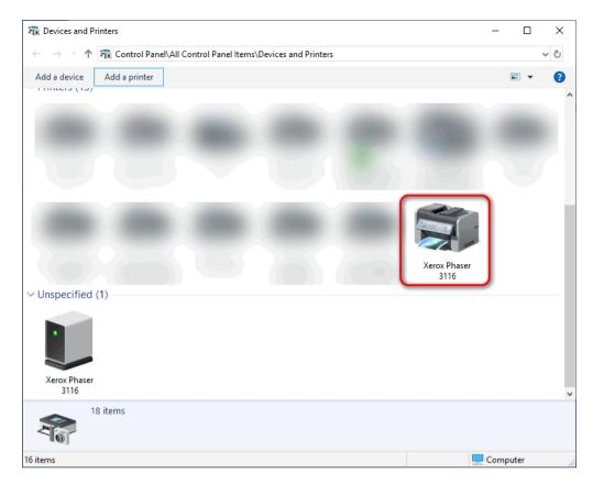
The **Xerox Phaser 3116** which shows up in the unspecified devices section, will continue to exist/show up, but no worries. The driver Xerox Phaser 3117 driver pipes data to the virtual printer port the printer is listening on (USBxyz) and it'll catch the data coming from the Xerox Phaser 1337 driver and print it.
