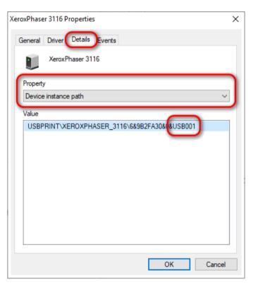
Take note of the last part, i.e. the **USBxyz** part (in this particular case, it's USB001, but it could also be USB002, USB003, USB004, etc.). That's the number of the virtual printer port for USB that the device is using. Write this info down or remember it. You can close all dialogue boxes now.
