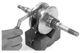
Set the crankshaft on V-blocks and measure the connecting rod big end radial clearance.
