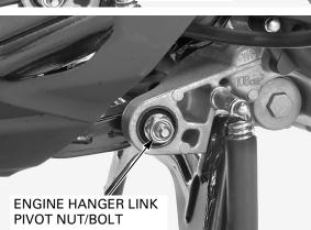
Remove the engine hanger link pivot nut (frame side).
