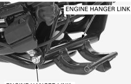
ENGINE HANGER LINK PIVOT NUT/BOLT
