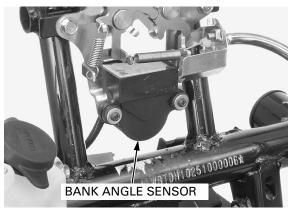
The center line of pendulum inside the bank angle sensor would be kept straight with the center line of vehicle when turning as the centrifugal force is applied to the pendulum, while it would be offset when the vehicle is overturned as the centrifugal force does not work.
