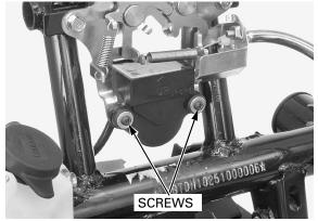
Connect the bank angle sensor 6P (Black) connector and clamp the bank angle sensor wire.
