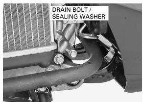
Reinstall the drain bolt with a new sealing washer onto the water pump cover.
