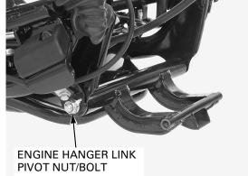
Set the engine to the frame by aligning the bolt holes of the engine and engine hanger link.
