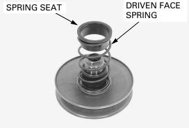
Install the driven face spring and spring seat.
