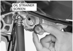
Make sure the O-ring is in good condition and replace it if necessary.
