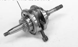
If the timing sprocket teeth are worn or damaged, check the cam chain, tensioner and cam sprocket.
