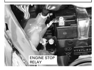
Place the bank angle sensor in normal position as shown, and turn the ignition switch "ON". The bank angle sensor is normal if the engine stop relay clicks, which indicates that circuit is closed.
