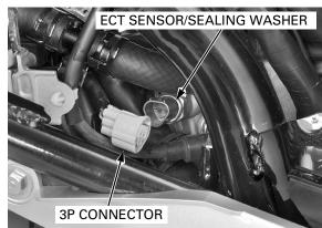
Always replace a sealing washer with a new one.
