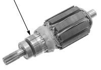
Check for continuity between pair of commutator bars. There should be continuity.
