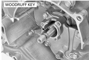
Remove the bolts and the stator base/water pump.
