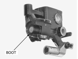
Remove the snap ring from the groove of the master cylinder. SNA TOOL:
