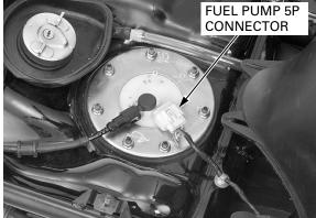
Remove the fuel pump mounting nuts. Remove the set plate and fuel pump unit from the Be careful not to fuel tank. damage the fuel level sensor float arm and pipe.
