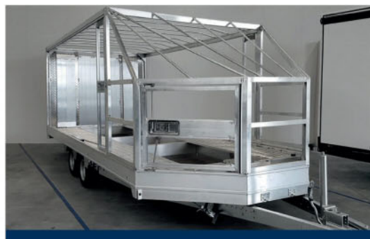
ALUMINIUM CONSTRUCTION Complete alloy chassis giving the system the lowest empty weight.
