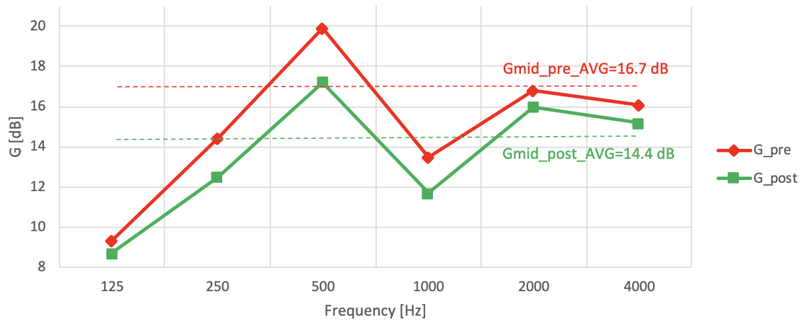
Figure 6 – Sound strength measurement results both before and after the refurbishment.
