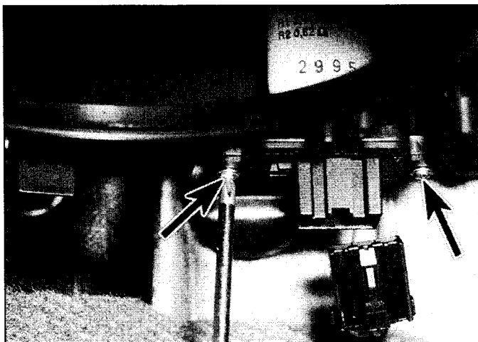
8.21a Remove the two securing screws (arrowed) . . .
