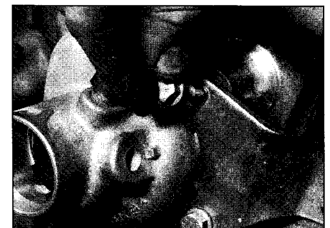
5.9a Unbolting the alternator upper bracket from the rear of the water pump
