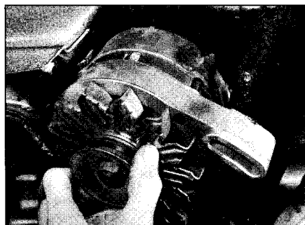
5.6b Removing the alternator (petrol engine)
