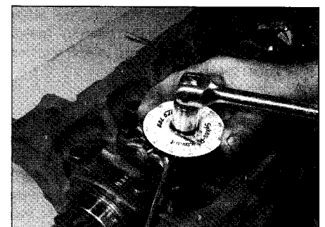
5.43b Angle-tightening the big-end bearing cap bolts (diesel engine)
