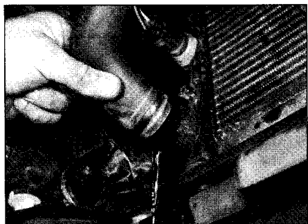
25.2 Disconnecting the radiator bottom hose to drain the coolant
