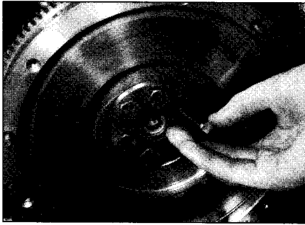
11.8b Inserting the flywheel bolts
