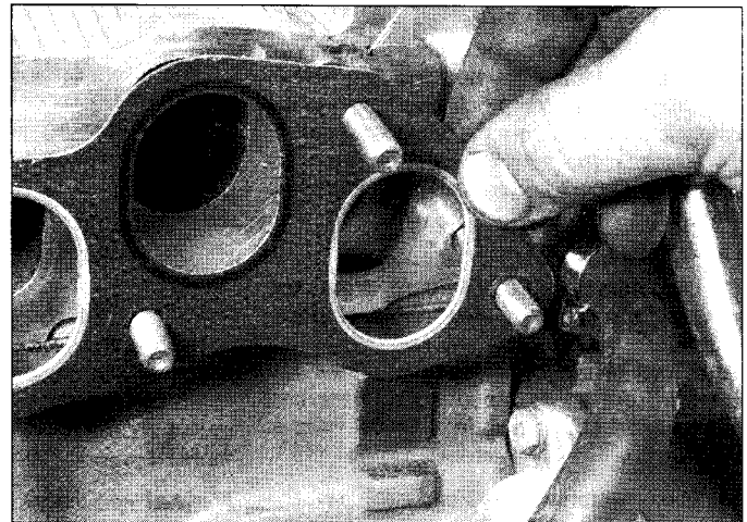
5.13 Removing the exhaust manifold gasket (diesel engine)
