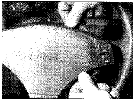
9.1 Prise the horn centre pad from the steering wheel hub
