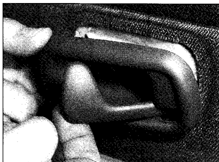
14.3b ... then prise out the door grab handle moulding
