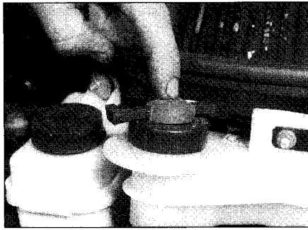
4.1 Depress the button on the top of the brake fluid reservoir cap
