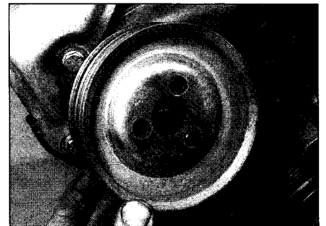
7.5b Lifting off the coolant pump pulley
