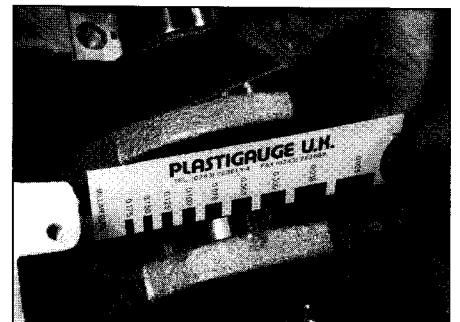
10.11 Use the special scale card to determine the main bearing running clearance
