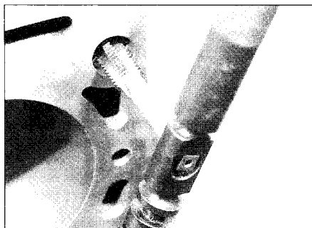
7.7 To clean the cylinder block threads, run a correct-size tap into the holes
