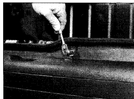
7.5 Remove the four retaining bolts from the upper edge of the bumper
