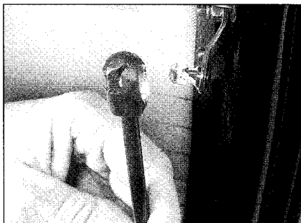
9.2b ... and then prise strut balljoint from the stud on the tailgate
