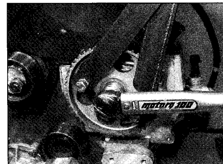
5.35 Tightening the injection pump sprocket bolt
