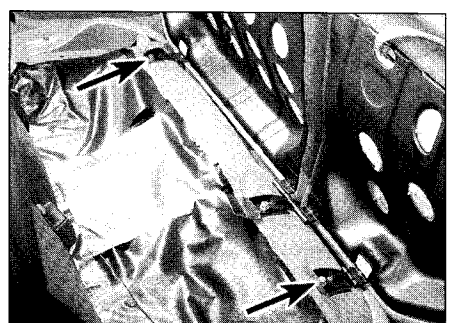
20.11 Remove the screws (arrowed) that secure the hinged brackets to the floorpan
