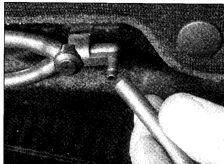
2.2b Disconnecting the washer tubing
