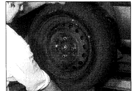
15.4 Rocking a roadwheel to check for wear in the steering/suspension components
