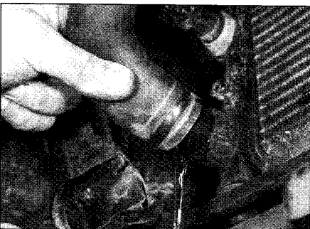
2.5 Draining the coolant by disconnecting the radiator bottom hose
