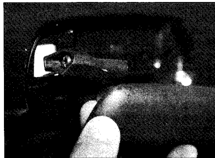
16.5b . . . and lift the handle assembly from the door
