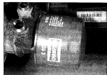
3.9 New oil filter tightened by hand
