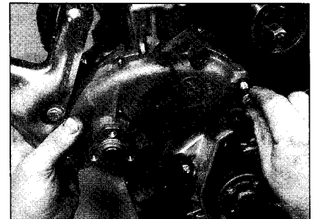
7.6c Removing the coolant pump assembly (diesel engined models)
