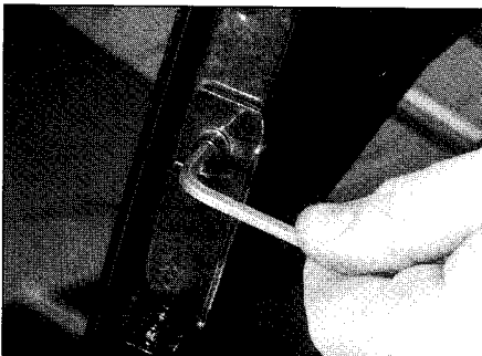
2.2a Unscrewing the bonnet hinge bolts
