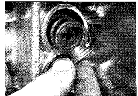
4.16a Removing the upper spring seat . . .
