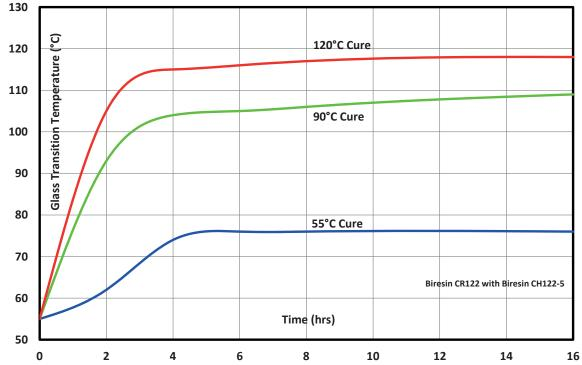
The test specimens were produced from 3 mm thick pure resin. Before the above postcuring, the samples were cured for 7 days at 23°C. When curing a composite part, the whole of the part (including the very middle of the laminate) needs to see the cure temperature.
