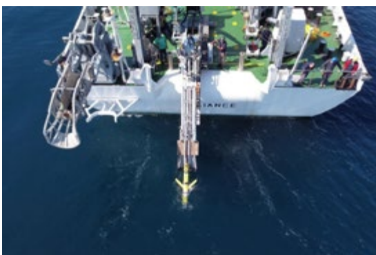
Autonomous underwater vehicle Slocum glider deployed from NATO Research Vessel Alliance during Exercise Robotic Experimentation and Prototyping augmented by Maritime Unmanned Systems 2021. Off the coast of Portugal, September 2021.
