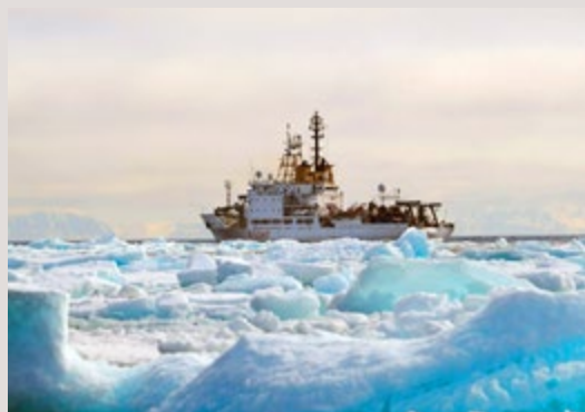
NATO Research Vessel Alliance on location in the Arctic during the Nordic Recognized Environmental Picture trial. The quietest ship in its class, the Alliance was designed to minimise noise radiating from the ship into the water, making it an excellent platform for sonar, acoustic devices testing and other types of research where a quiet undersea environment is essential. Arctic Ocean, June 2021.
