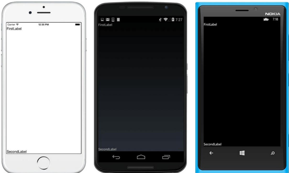
Figure 3-12. secondLabel placed at the bottom of the screen with y set to 1
