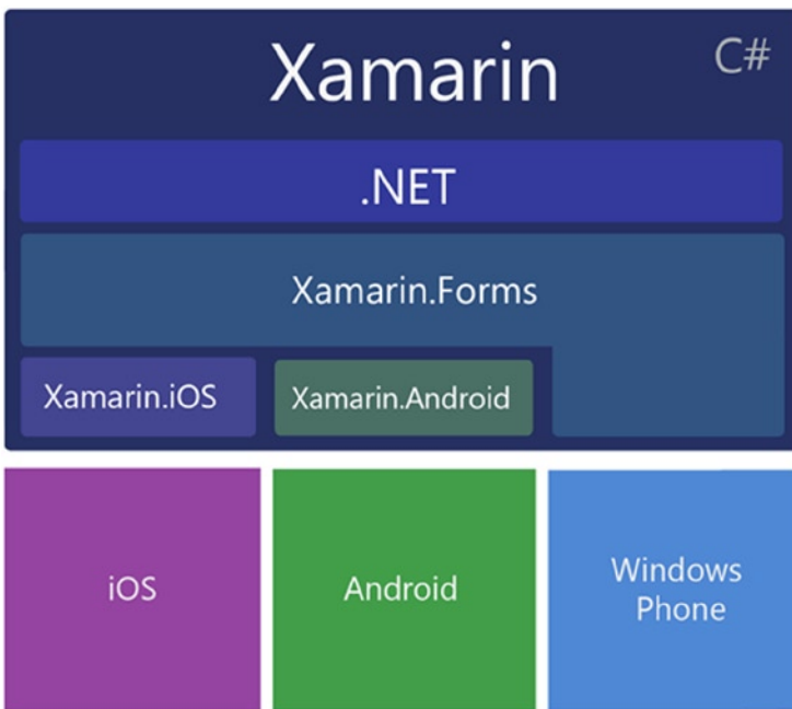
Figure 1-1. Xamarin C# libraries bind to native OS SDKs as well as .NET
