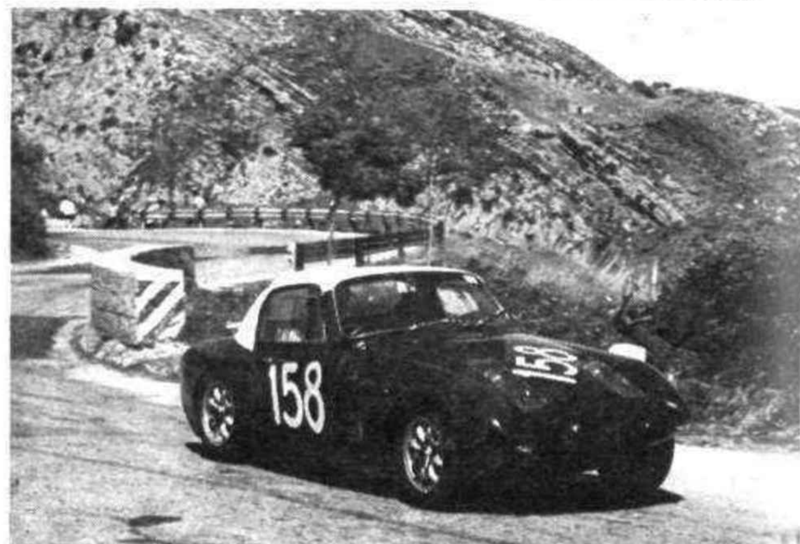
TARGA FLORIO SPECIAL.—Jack Wheeler and Martin Davidson built this one-off Sprite especially for the event, featuring Lotus Elan suspension with the backbone grafted onto the Sprite chassis. Unhappily the suspension did not go the distance.
