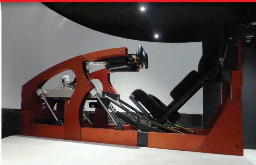
ABOVE & BELOW The Evolution II can transform from a Formula 1 driving position (above) into GT (below) at the touch of a button
