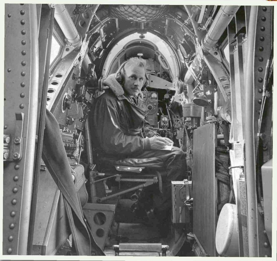
ABOVE: Although this photo was taken in pre-war Britain, it clearly demonstrates the limited space in the fuselage of a Wellesley. To retain the strength of the geodetic construction, no bomb bay was carved out the fuselage; instead, all bombs were carried in large panniers mounted under the outer wings. AEROPLANE
