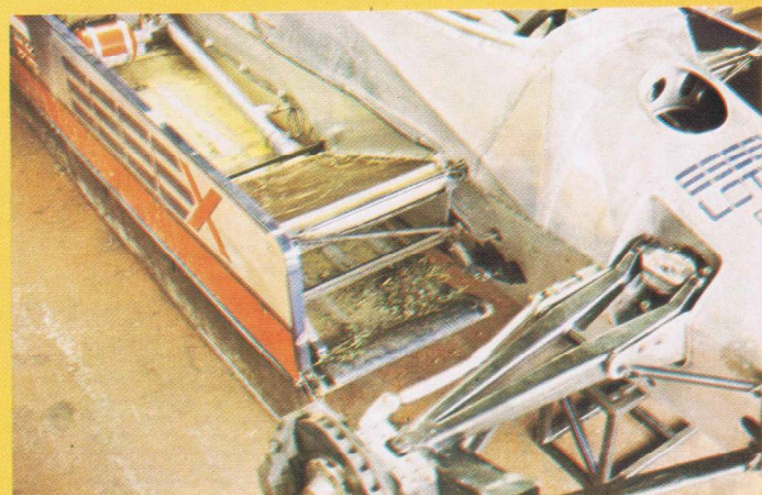
1 - Upper part of the chassis now strengthened, but a sidepod came loose on Saturday.
