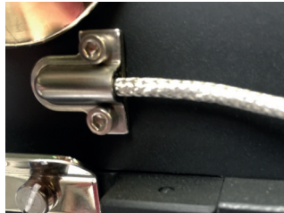
Temperature sensor Double read-out 3mm
