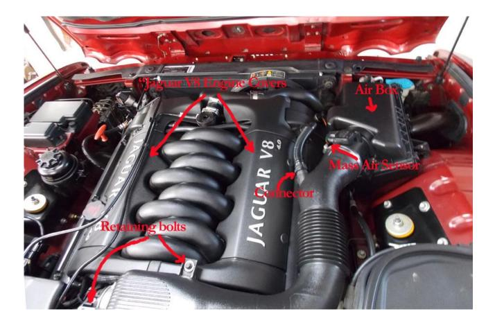
7) De-pressurize the fuel rail system by removing the small blue screw cap located at the right/passenger rear of the fuel rail, and depress the Shrader valve. Have a clean rag ready to soak up any gasoline. Replace the blue cap.
