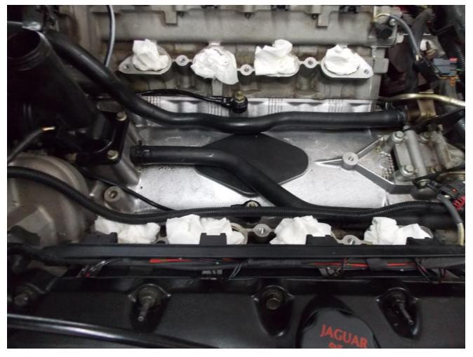
20) I recommend you also replace the plastic 3-way connector, NNE3944BA, at this time. Be careful disconnecting the main feed to the 3-way connector, you do NOT want to break the retaining clips on that plastic main feed connector!
