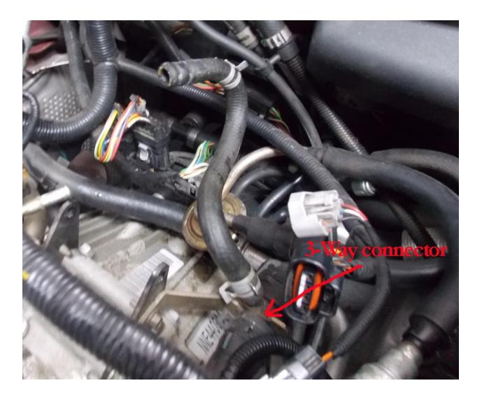
21) Once the intake valley has been cleaned, the two heater hoses have been replaced, and the 3 way connector has been replaced. If you still have the original plastic thermostat housing, now is the time to replace it with a metal version. (And also replace the thermostat if it has not been replaced recently)
