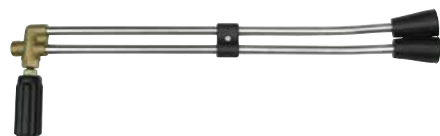
Double lance with regulator knob max 250 bar: for high/ low pressure regulator, max temperature 150° C, for gun M 22 (nozzles 1/8" not included)
