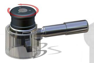
3. After that, give the **Bravo Distributor & Leveler** a quick spin, 2 or 3 revolutions counterclockwise, and so the vertex in the bottom of the piston will level out the coffee in the filter basket, thus making it ready for tamping.
