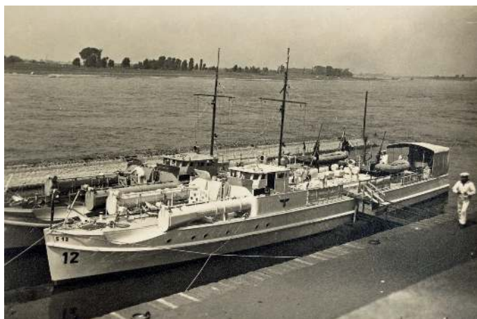
■ Forerunner of the classic S-Boot design of the Second World War, this was the S.2, one of the vessels developed in the late 1930s. With a petrol engine, later developments saw S-Boote fitted with powerful diesel engines which reduced the fire risk.
