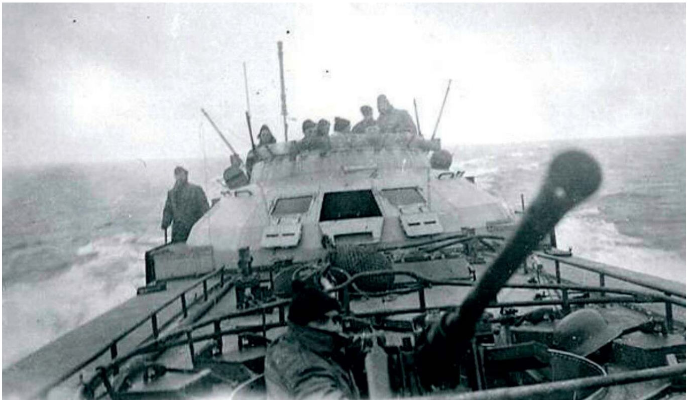
■ A view across the 2cm Flak 38 gun towards the fully armoured bridge section (Kalottenbrücke) which was introduced with S-100.
