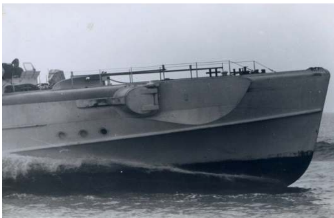
■ The bow of the S-27, showing the port of one of her torpedo tubes.
