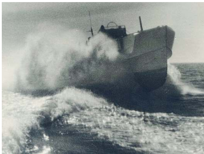
■ At speed, as Captain Peter Scott RN later observed, the bow spray from the S-Boote rose up and passed over the vessel, leaving the crew dry. The opposite was the case on British MTBs!
