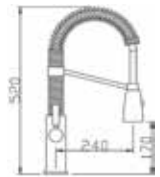
Code : T-8000A Single Lever Kitchen Sink Mixer * Spring Flexi Spout with Sprayer * Dual-modes Spray * 35mm cartridge
