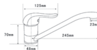
Code : T-4036 Single Lever Pillar Sink Tap * with Swivel Spout * 40mm Cartridge
