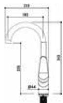
Code : SDC-180-CR Single Lever Sink Tap * with swivel spout * 35mm cartridge
