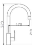
Code : SBC-2528 Single Lever Sink Tap * with swivel spout * 25mm cartridge
