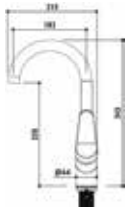
Code : SDM-180-CR Single Lever Sink Mixer * with swivel spout * 35mm cartridge
