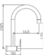
Code : SBC-2528W Single Lever Sink Tap * with swivel spout * 25mm cartridge
