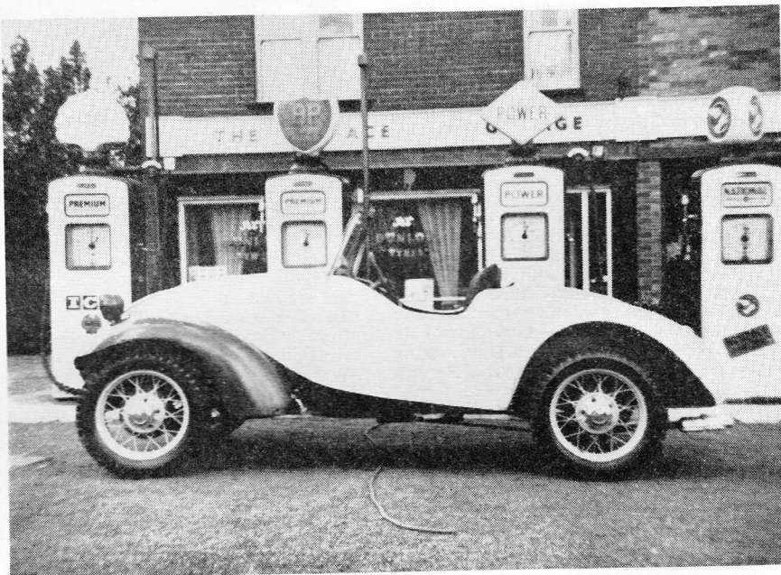
THE X100, a Y Model Ford stripped to the chassis and fitted with a special body built by Trevor Taylor and his brother Mike. The car was shown on a television programme and was used in a few sprints and hill-climbs.
