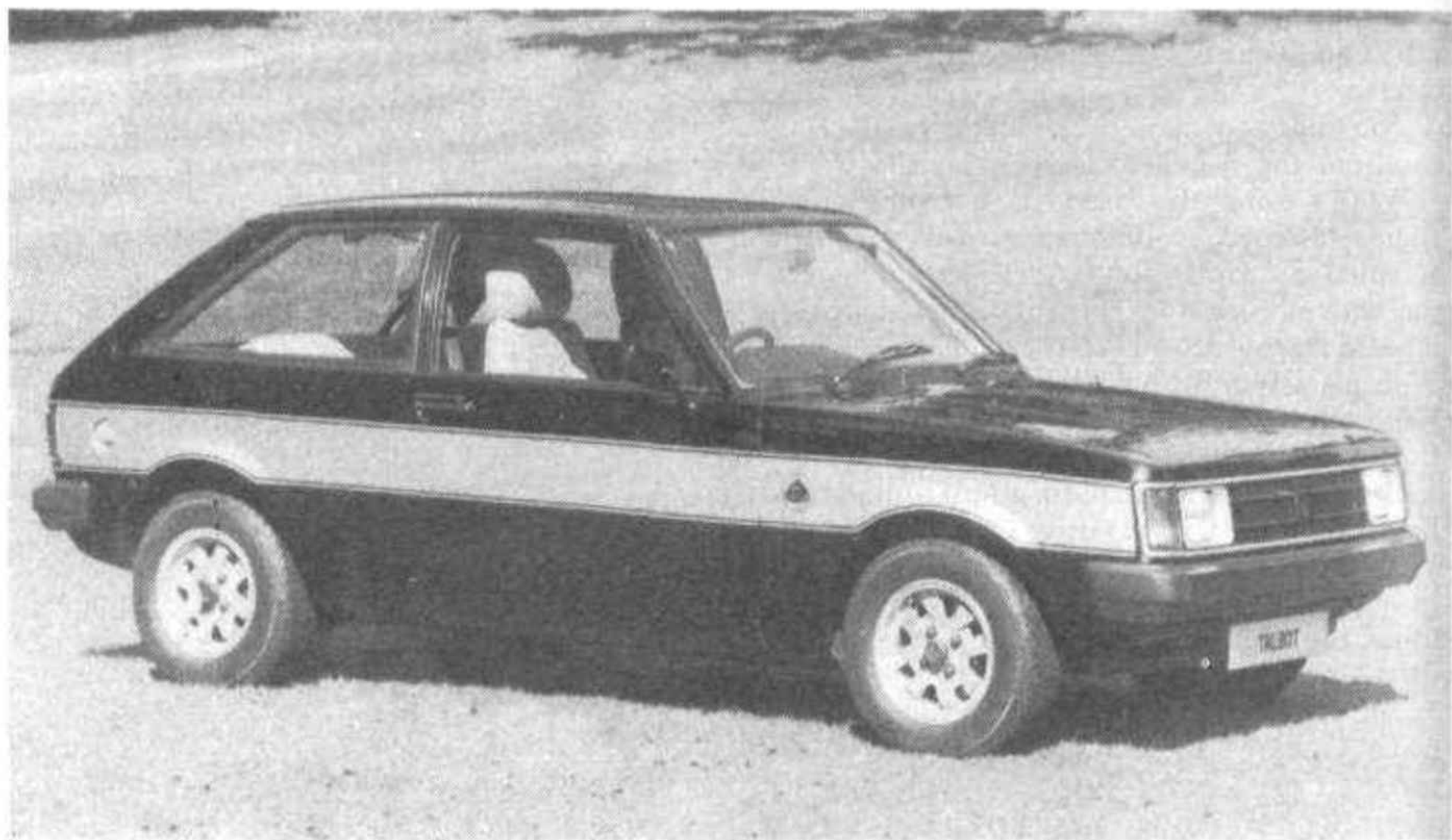
Any colour so long as it is black (with silver side-stripes). This pre-production Talbot Sunbeam Lotus is missing its standard fog lights, mounted above the bumper.
