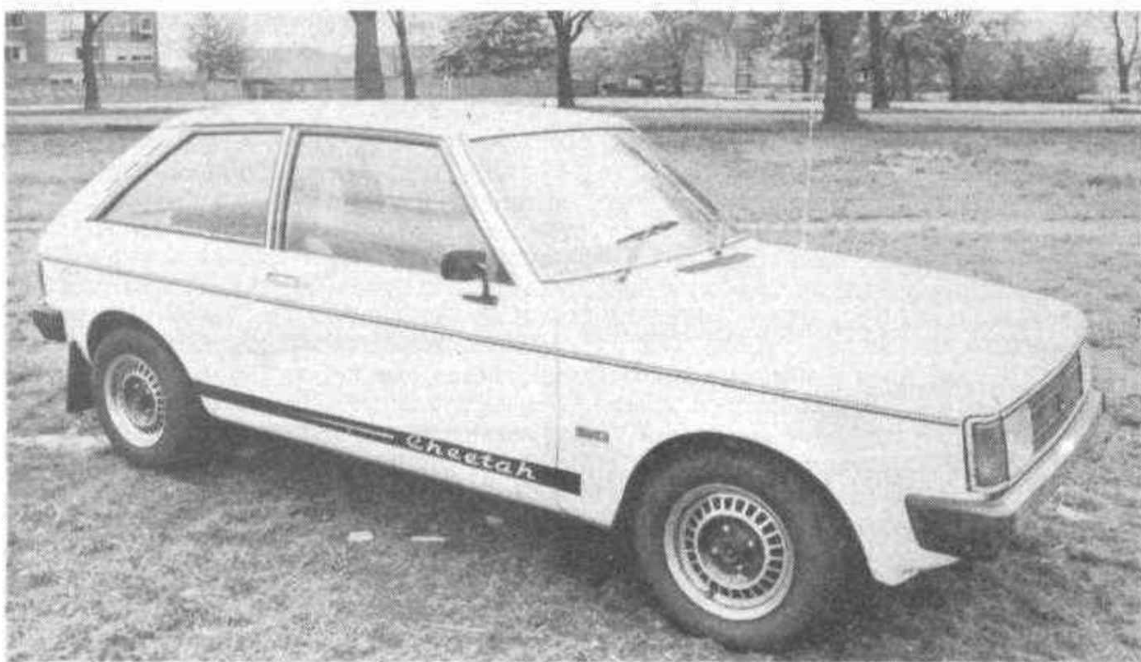
Alloy wheels with 6 in. rims are standard on the Cheetah, but the Sunbeam body is unmodified apart from appropriate badging.
