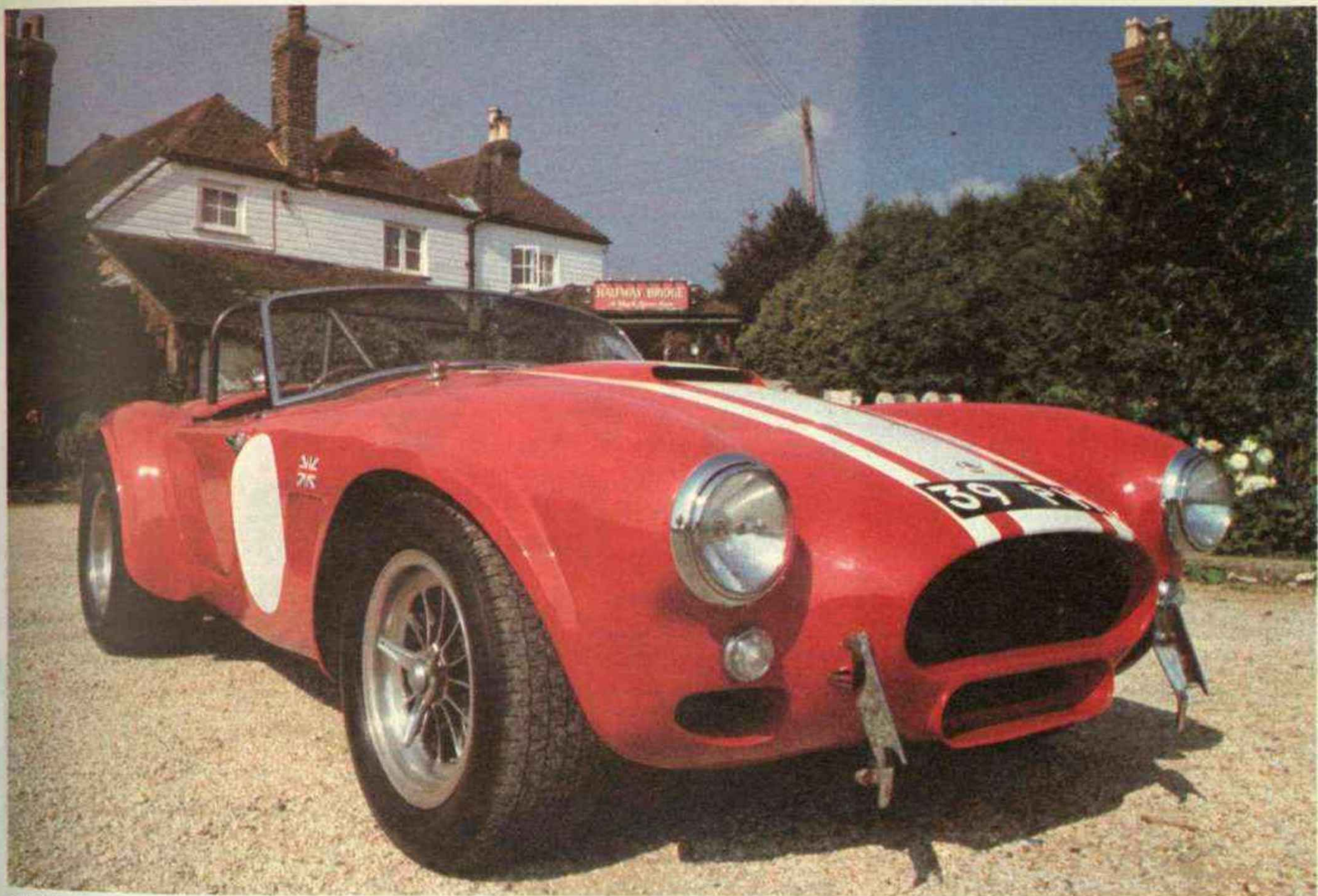
The Willment Cobra made famous by Jack Sears in 1964 as it is in 1979, impeccably restored by owner Nigel Hulme. The front protruberances are locating lugs for the quick lift jack. Major items visible, like the body, Halibrand wheels and roll-over bar are original. Willment ran the windscreen at a sharper angle.
