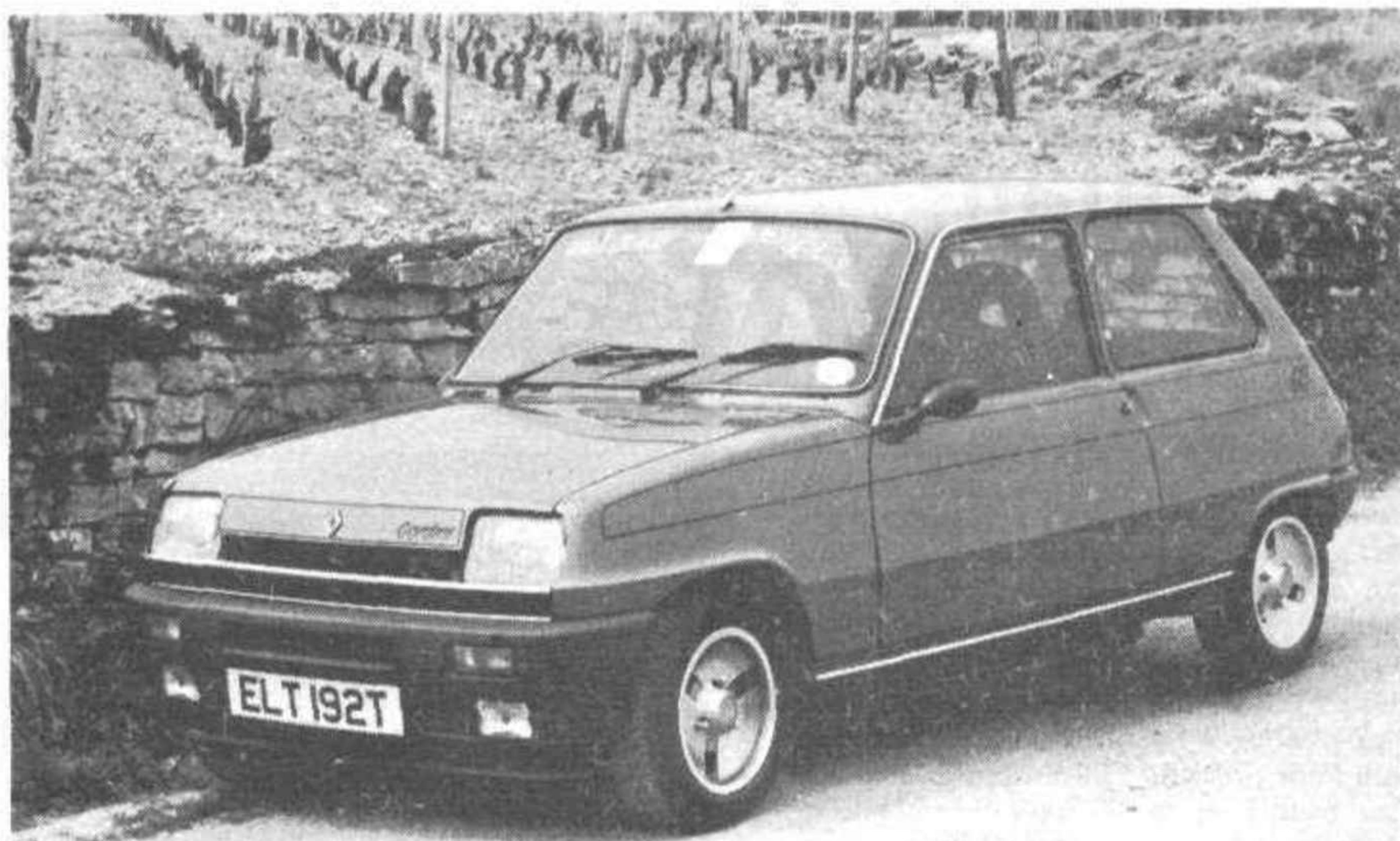
A front-spoiler and attractive alloy wheels make the Gordini easily distinguishable amongst the other Renault 5s.
