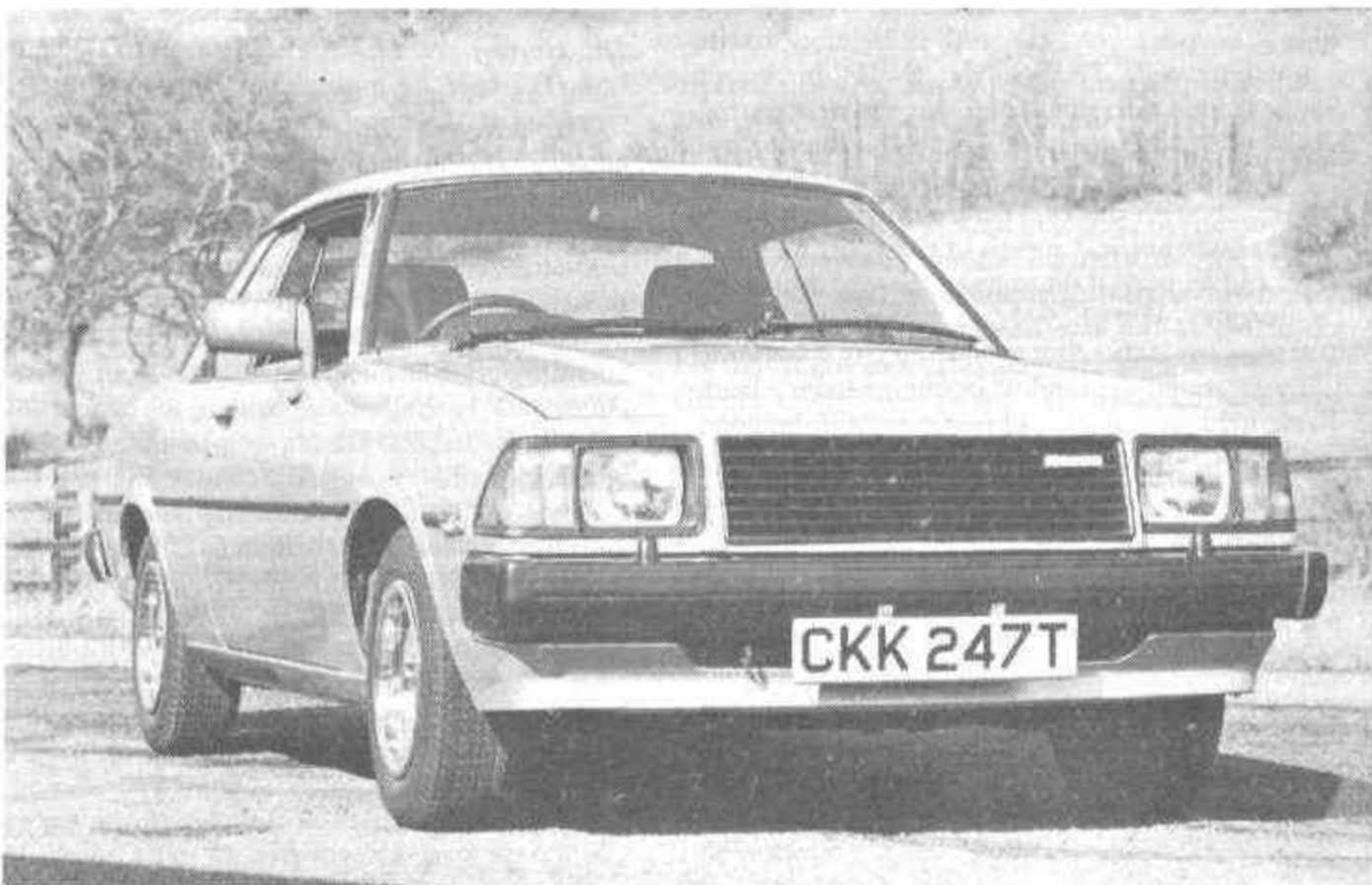
The low frontal area is an aid to good performance. Note the high-pressure washers for the Cibicé halogen headlamps.
