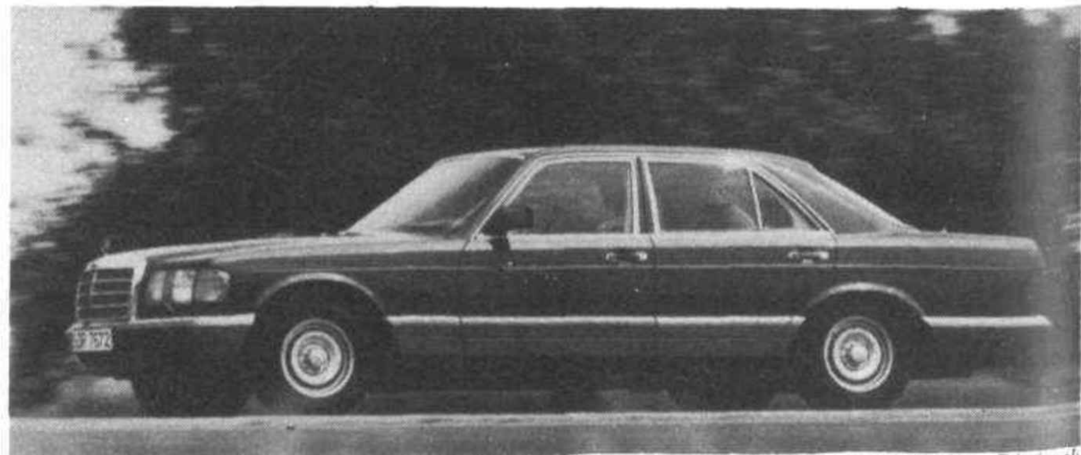
Mercedes Benz's new S-class range made its debut at the Frankfurt Motor Show in September. Distinctly wedge-shaped, its lines nevertheless owe a lot to the present S-class saloon, which continues in production for the time-being. Innovations include a wind-cheating body with a resistance value 14 per cent more efficient than before, and light alloy V8 engines of 3.8 and 5-litres in addition to the current in-line, 2.8-litre, twin cam six cylinder.
