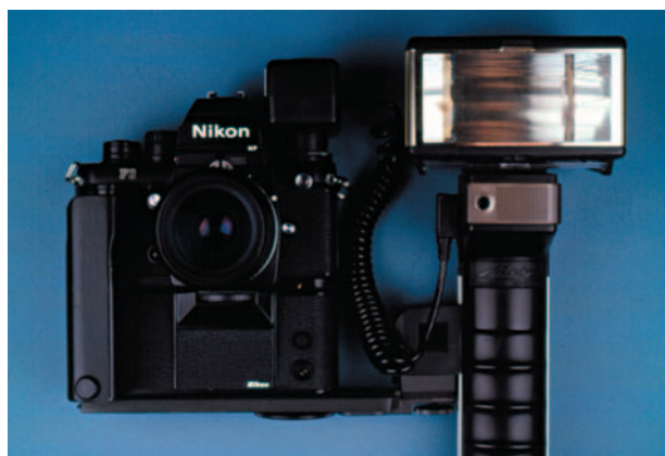
FIGURE 26.1 35mm SLR camera with a motor winder and electronic flash.
