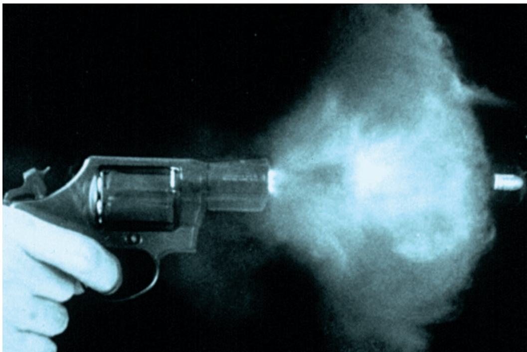
FIGURE 22.1 A high speed flash photograph of a revolver at the instant of discharge. Large volumes of gas are emitted from the muzzle and also a certain amount escapes from the cylinder gap. The residues from the primer are sought in GSR sampling. (Photograph courtesy of A/Prof Gale E. Spring-Royal Melbourne Institute of Technology University).
