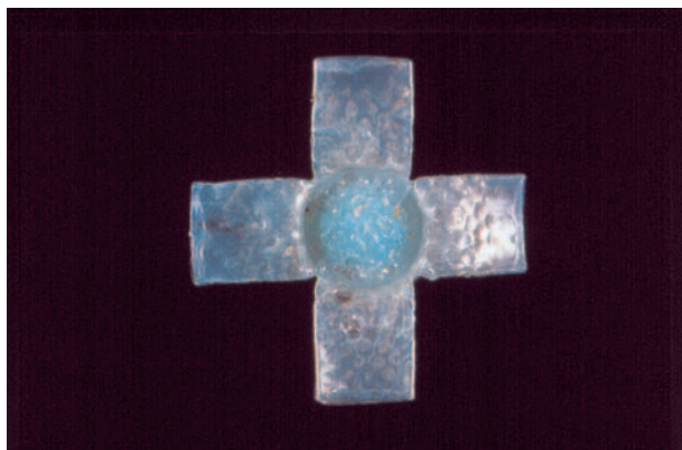
FIGURE 11.19 A fully opened piston. Note the radial separation and pellet indentation. Always retrieve and submit the piston/wad as evidence.
