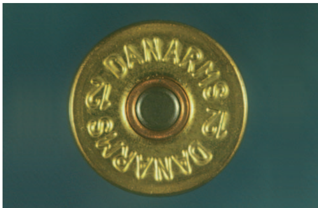
FIGURE 2.6 Base of brass head showing manufacturer's stamp, gauge and primer in situ.
