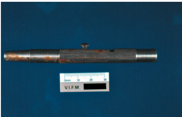
FIGURE 16.5A Home made pen gun accommodating a .22 long rifle cartridge.
