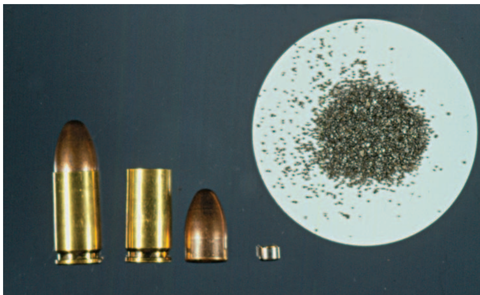
FIGURE 3.4 The components of a typical 9 mm cartridge. From left to right: intact round, cartridge case, fully jacketed round nose projectile, primer cap, and propellant
