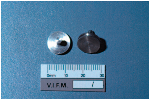
FIGURE 22.3 Small stainless steel studs with adhesive surfaces are used to pick up the fine GSR from the skin of the proposed firing hand.
