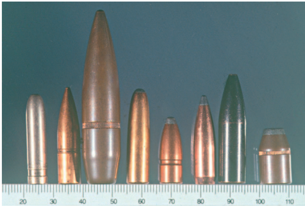
FIGURE 4.4 A selection of projectiles. From left to right: (military) round nosed, Spitzer and Boat tail (hunting), round nosed soft point, Spitzer soft point, semipointed soft point, Spitzer hollow point, and semijacketed hollow point.
