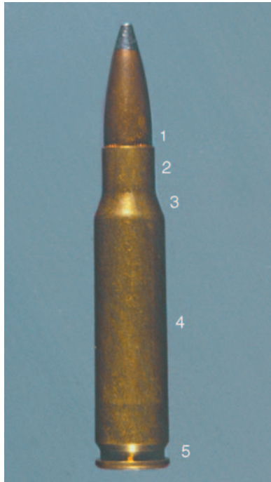
FIGURE 4.2 A typical centerfire round. .308 caliber cartridge with a soft point Spitzer projectile.
