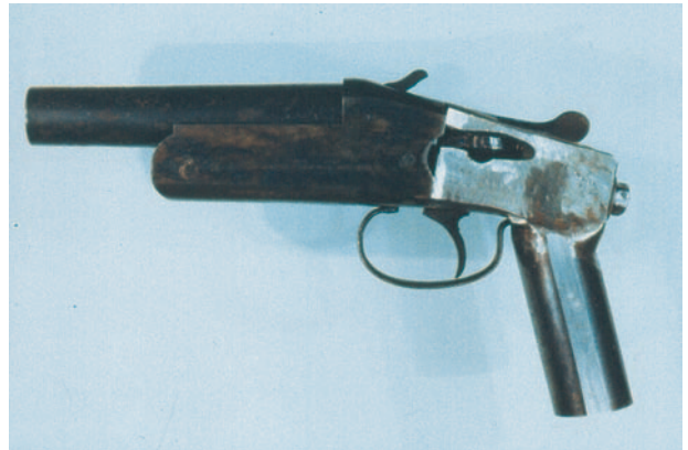
FIGURE 16.6A Hybrid gun. Modified 12 gauge shot gun accommodating a .38 caliber pistol cartridge. A grip has been fashioned from a length of pipe welded to the action.
