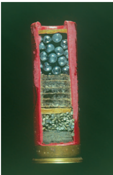
FIGURE 2.3 An opened shotgun cartridge of older design showing the brass head, propellant, over powder card, wadding, projectiles, and cap.
