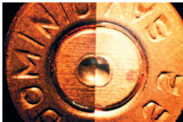
FIGURE 22.10 A split image view of a questioned and comparison cartridge baseplate. Careful attention is paid to the pattern imparted by the firing pin and ejector mechanism.
