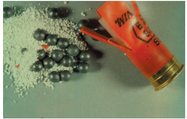
FIGURE 2.11 Opened shot shell showing piston (in situ), lead balls, and inert filter.
