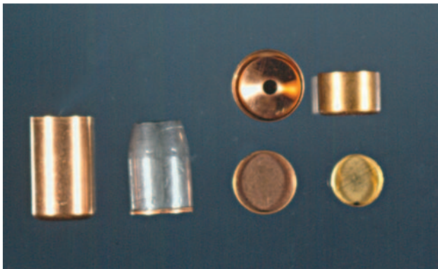
FIGURE 3.6 Gas checks are metallic plates or cups that protect the base of the projectile from the intense thermal effects at the instant of discharge. A representative sample is shown here.
