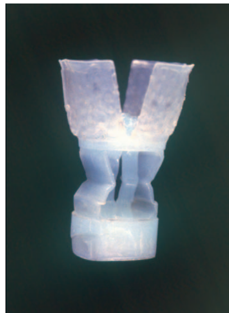
FIGURE 2.8 Spent piston showing pellet indentation.
