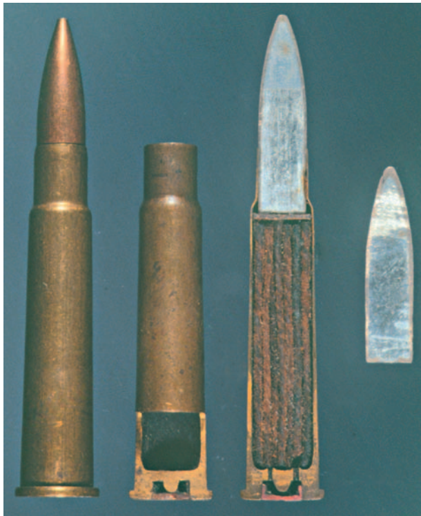
FIGURE 4.3 The components of a typical centerfire round. The .303 British. Note cartridge case, primer, flash hole, propellant, and projectile.
