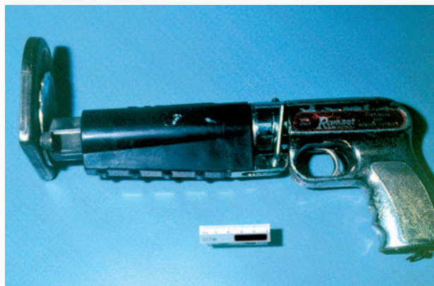
FIGURE 14.1 The nail gun used as a weapon of suicide. The nail gun was powered by a .22 caliber cartridge.
