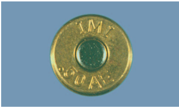
FIGURE 3.5 Head stamp. The .50 AE showing the manufacturer's stamp and caliber.
