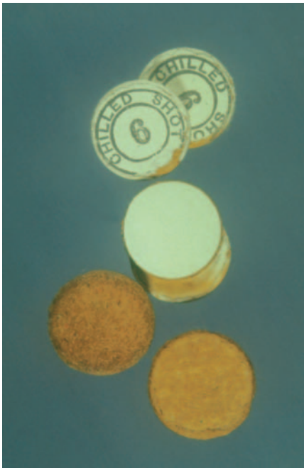
FIGURE 2.10 Cardboard wadding and capping as may be found in older style shells or in reload cases.
