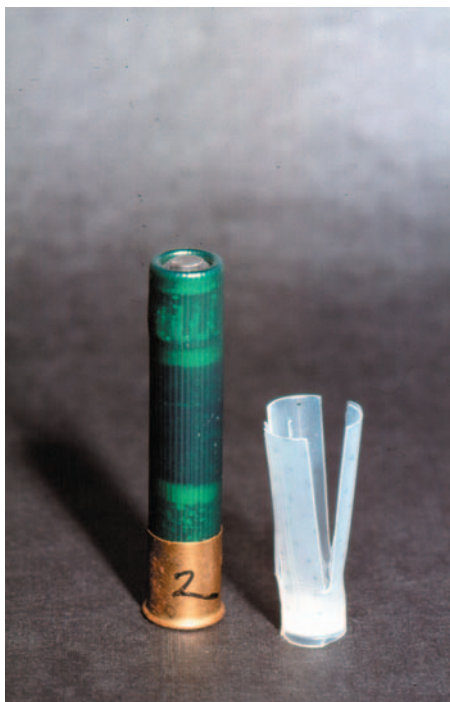
FIGURE 2.15 The .410 cartridge. This caliber of shot shell may contain a plastic piston with three leaflets or conventional cardboard discs.
