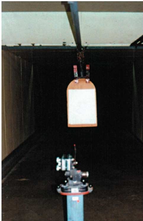
FIGURE 22.12 A modern test fire range with mobile overhead target and remote firing mechanism.
