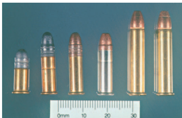
FIGURE 5.1 The .22 rimfire family from left to right: .22 Short .22 Long .22 Long rifle .22 “Stinger” .22 Magnum (with FMJ and hollow point projectiles).
