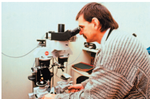
FIGURE 22.9 A firearm examiner using the comparison microscope. The questioned and comparison projectile or cartridge cases can be individually mounted, rotated, and viewed through the eyepiece in a split image mode.
