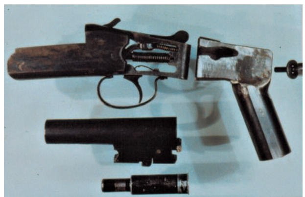
FIGURE 16.6B Action exposed. Note the sleeve like adaptor reducing the internal breech diameter from 12G to .38 cal. (bottom of photograph).
