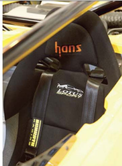
Nestled beneath the FIA-spec rollover structure is a HANS-approved carbon fibre seat fitted with a Schroth six-point harness
