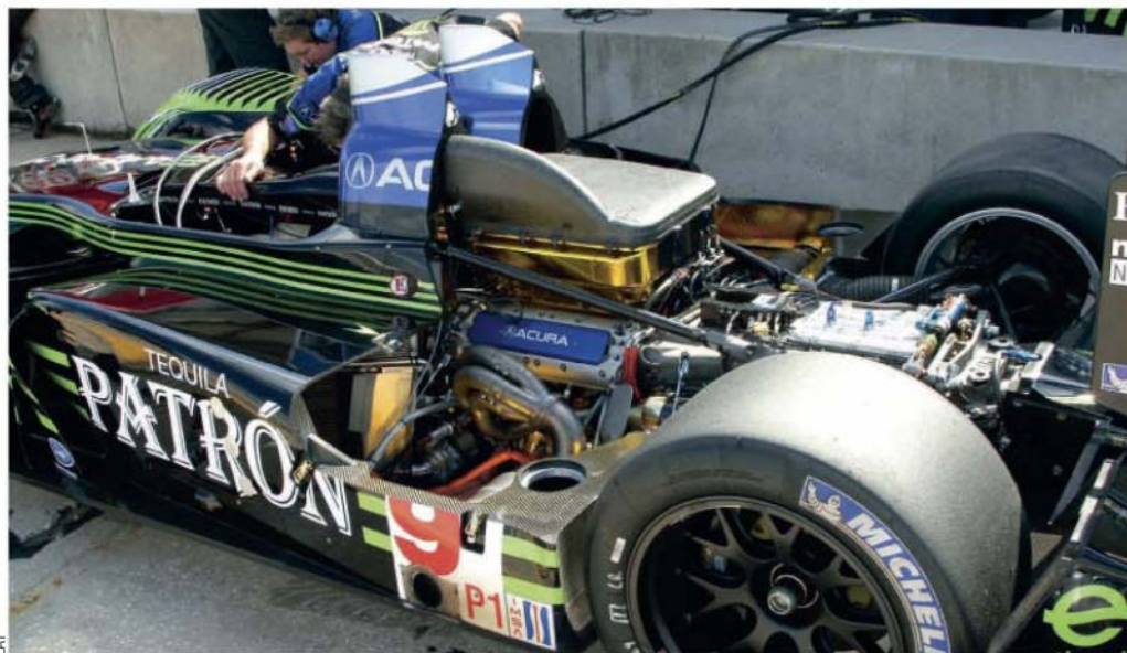
Chassis development centred on the idea of using the wider rear tyres on the front to maximise contact patch area
