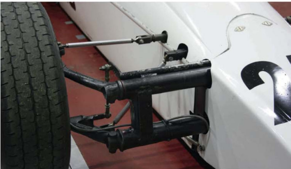
Formula Vee racercars use modified VW Beetle front suspensions, with transverse leaf stacks that work in torsion
