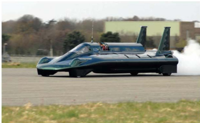
With 12 boilers and three megawatts, the British Steam Car aims for a century-old record
