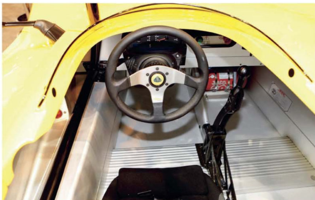
Cockpit shot of GT4 version shows gear shifter for ZF sequential transmission, Lifeline plumbed-in fire extinguisher system and, just visible on the left, a panel that includes a selector for the adjustable traction control system
