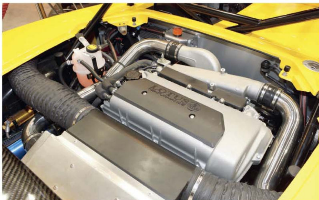
The 2-Eleven also uses the Toyota 2ZZ-GE engine, only this time tuned by adding a supercharger and intercooler
