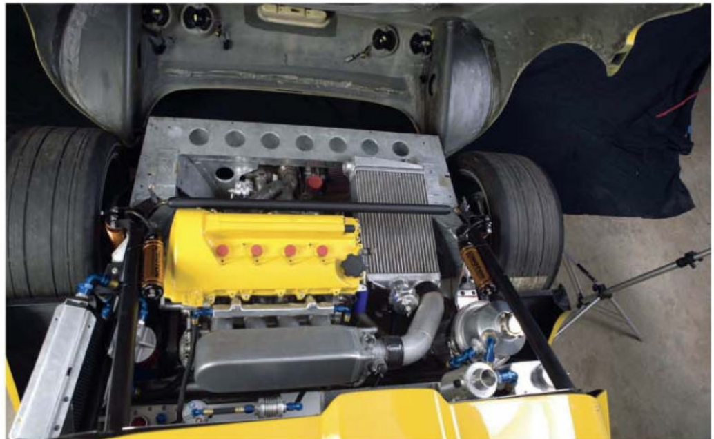
Exige S engine is a turbocharged version of the road car's Toyota 2ZZ-GE in-line four, with MoTeC management
