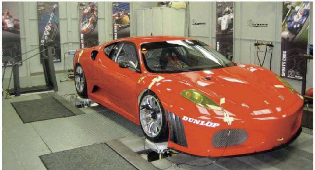
Ferrari F430 GT2 car on Multimatic four-post rig, which incorporates two pneumatic actuators to add aero loading
