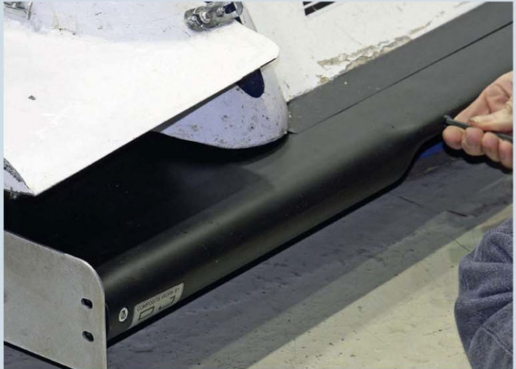
A selection of interchangeable leading edges made evaluating different length splitters possible
