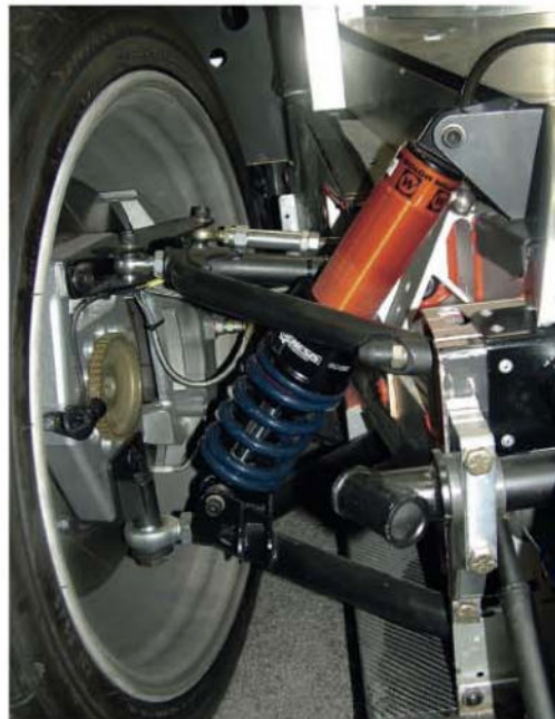
Front uprights were re-manufactured to accommodate 18in wheels and the ride height specified by the series organisers but otherwise the race version retains essentially the stock Exige road car's suspension geometry
