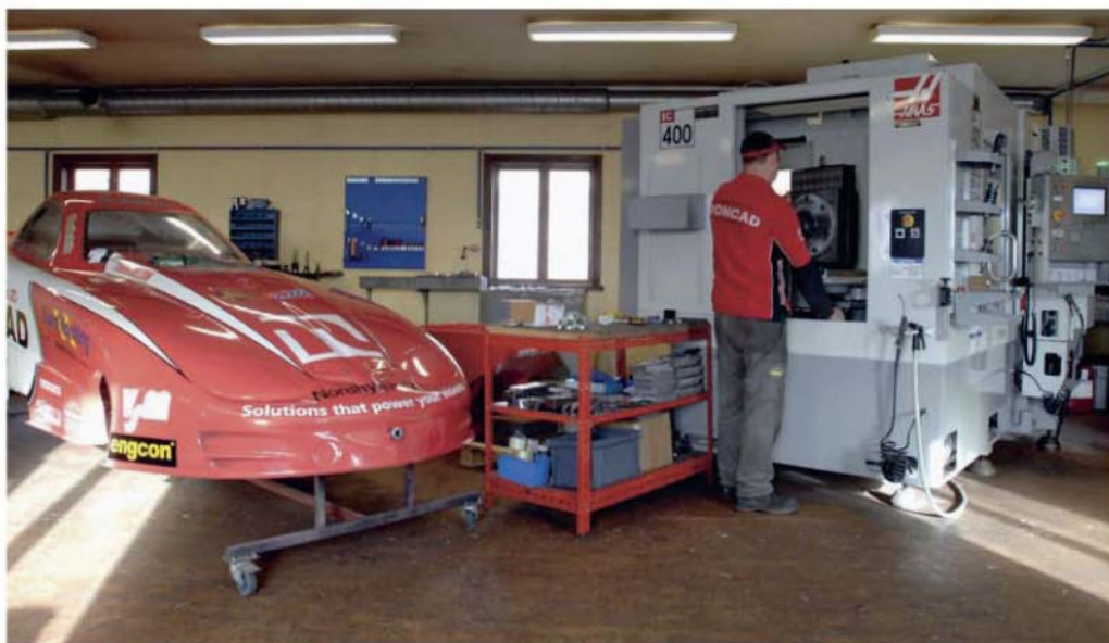
The Haas EC400 machining centre where the team produces its own titanium-based clutches for its Funny Cars
