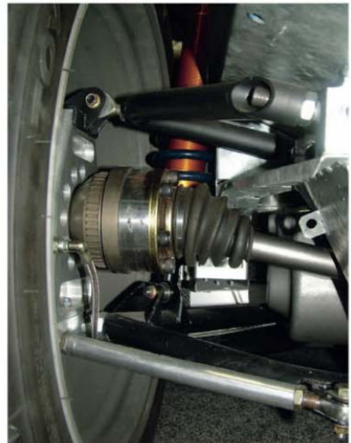
Front uprights were re-manufactured to accommodate 18in wheels and the ride height specified by the series organisers but otherwise the race version retains essentially the stock Exige road car's suspension geometry
