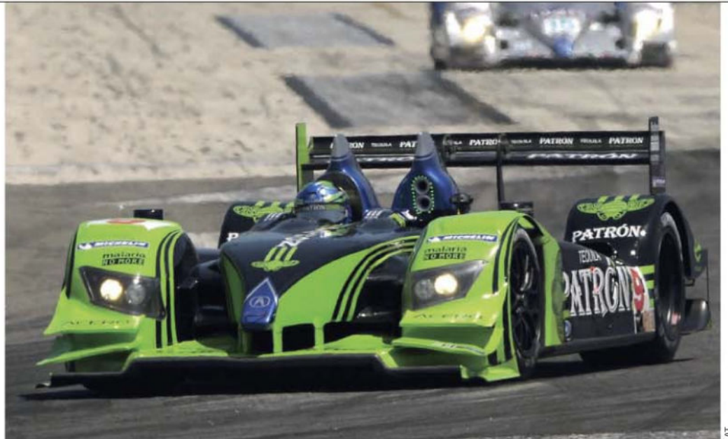
Using the wider tyres up front meant a complete re-design of the front suspension and aero, resulting in the adoption of an F1-style 'zero keel' approach
