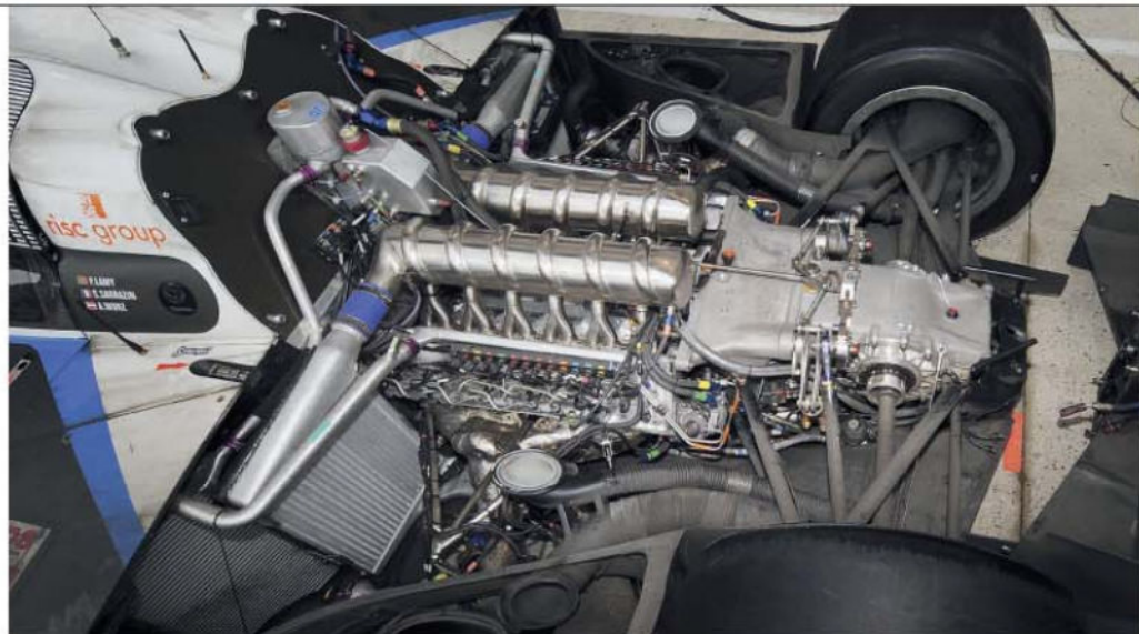
Conversely, a pair of short, horizontally mounted torsion bars are housed in the bellhousing at the rear of the Peugeot 908 HDi FAP LMP1
