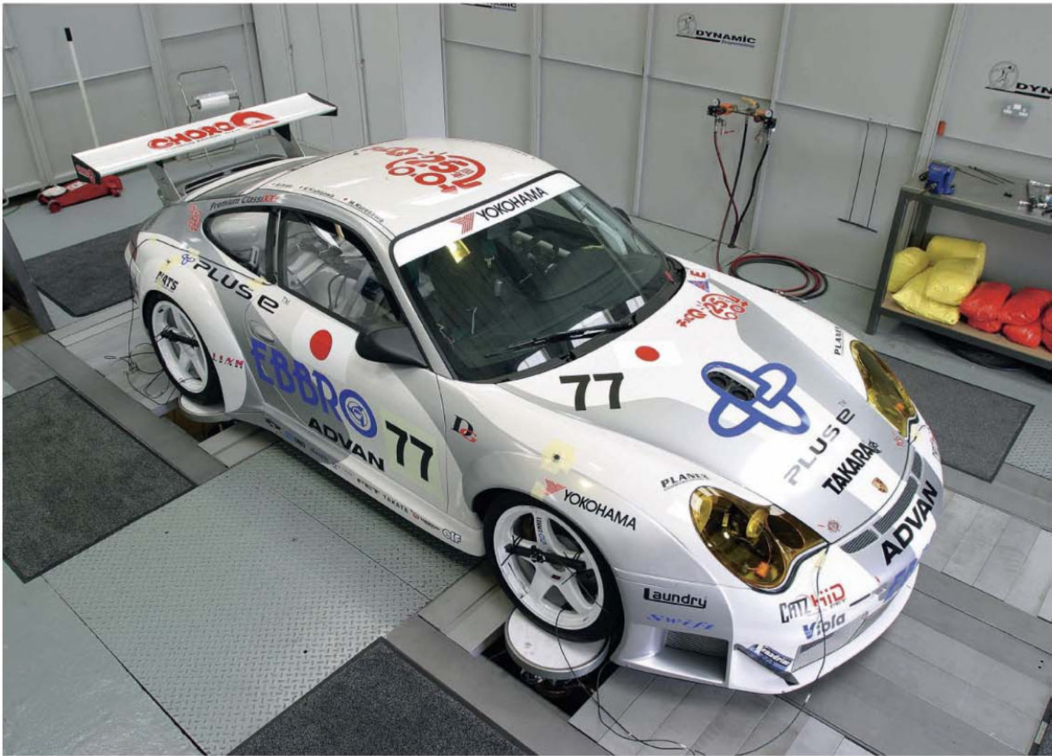
Williams always prefers to work with real racecars in race trim as items such as anti-roll bars, which may be left off, can have a dramatic effect on set up
