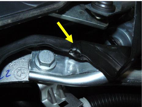
Install a longer strip (approx. 60 cm) of the same 6 or 7 mm diameter Butyl sealing tape onto the sealing surface of the center partition, in place of the original seal.
