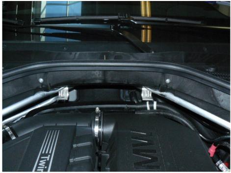
Required preliminary work: Remove the hood seal and the left and right microfilter housing covers.
