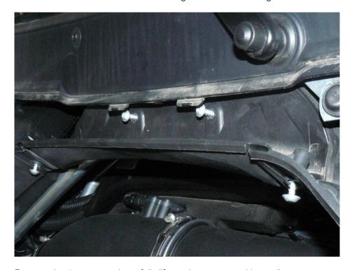
Remove the 4 screws and carefully lift out the center partition wall.
