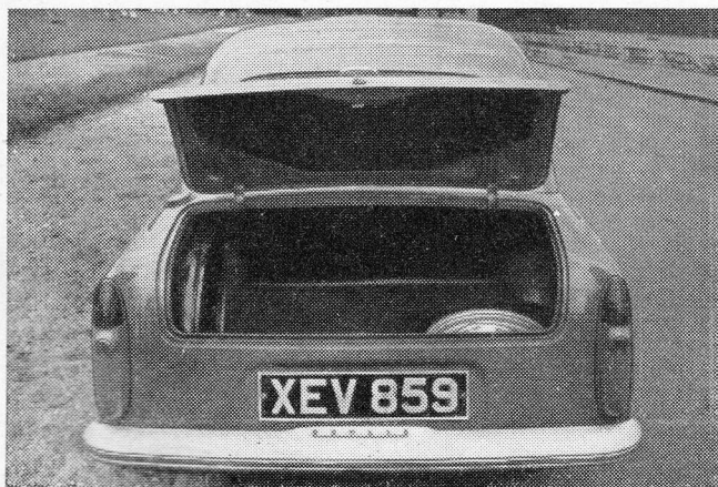
ONE advantage of the modern body styling on the Ford Anglia is the provision of a particularly capacious luggage boot. It is 18 inches deep, more than two and a half feet long, and almost four feet wide.
