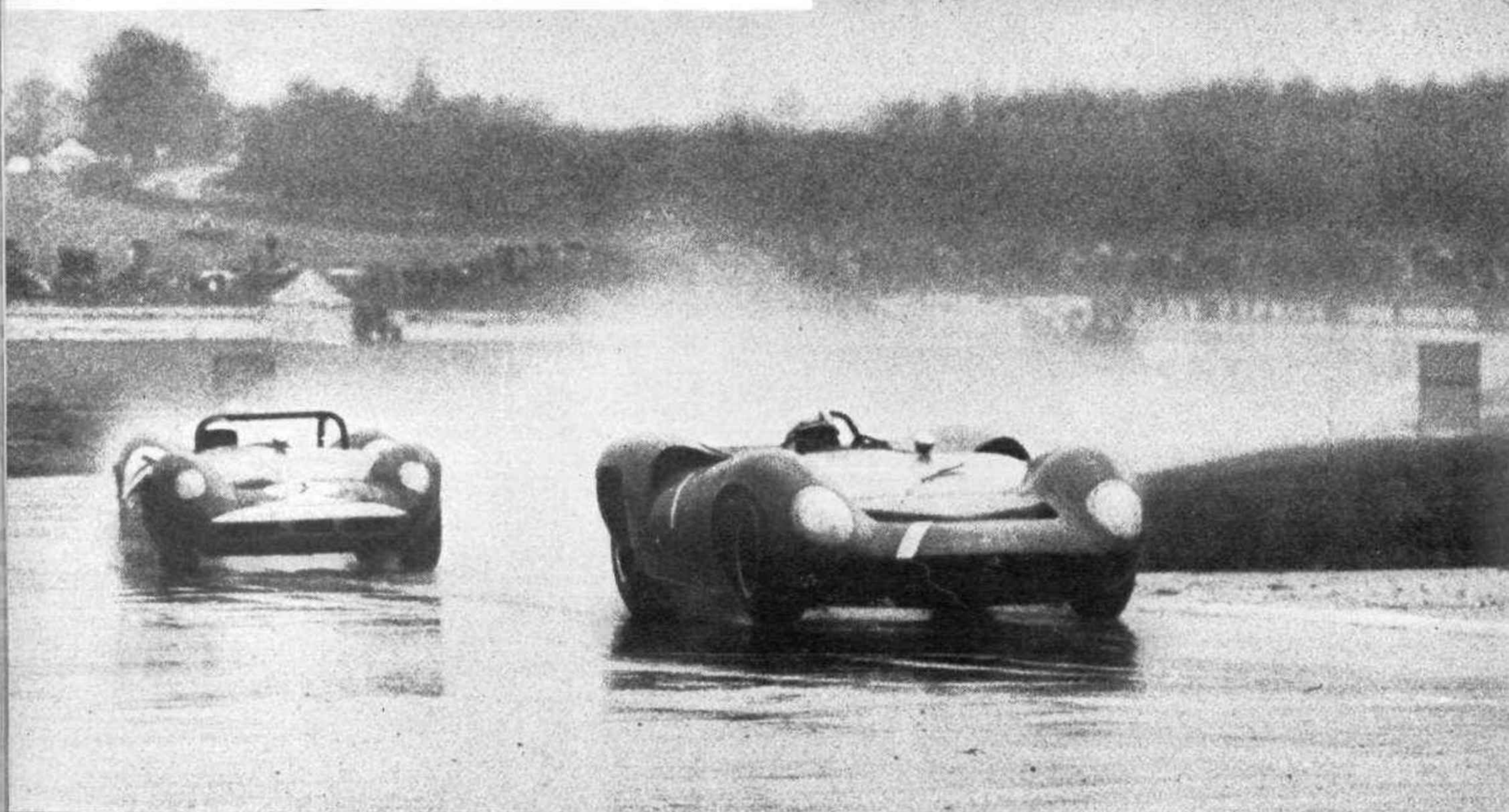
TEN LITRES IN THE WET. —Surtees (Lola 70 now fitted with a 5.3-litre Chevrolet engine) leads Clark (Lotus 30—4.7-litre Ford) through Abbey Curve. They both experienced spins but Clark was on Dunlop R7 tyres to Surtees' R6 and appeared to suffer less from aquaplaning as a result. Clark was leading when the race was abandoned. ▲
