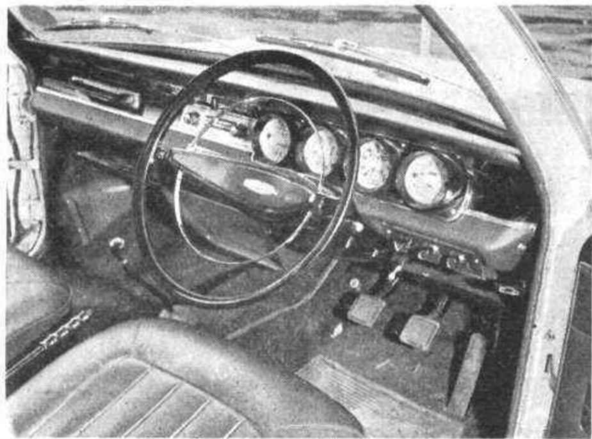
The conventional but comfortable and well-appointed "office" of the latest Vauxhall VX 4/90. Note the three differently-shaped knobs for lamps, spot-lamps and wipers/washers, all convenient to the driver's right hand.
