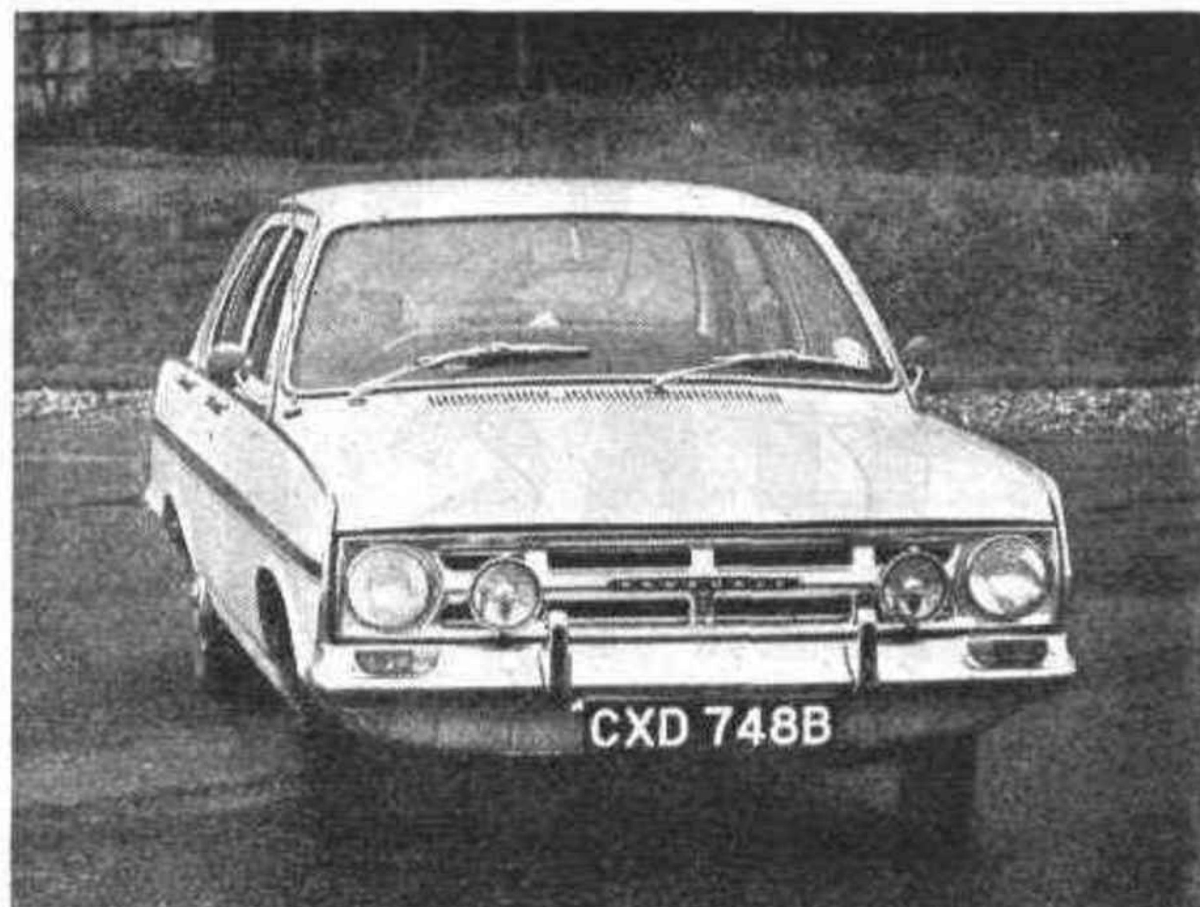
The latest Vauxhall VX 4/90 from Luton has a rather crude radiator grille which was apt to draw forth remarks about "Dinky Toys." This view shows the tumblehome of the side windows, which gives increased interior accommodation.
