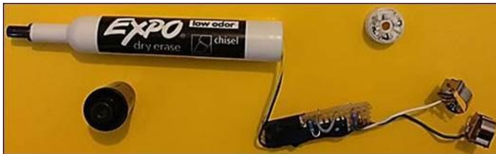
Figure 1.11: A marker converted into a hotel lock opener.
