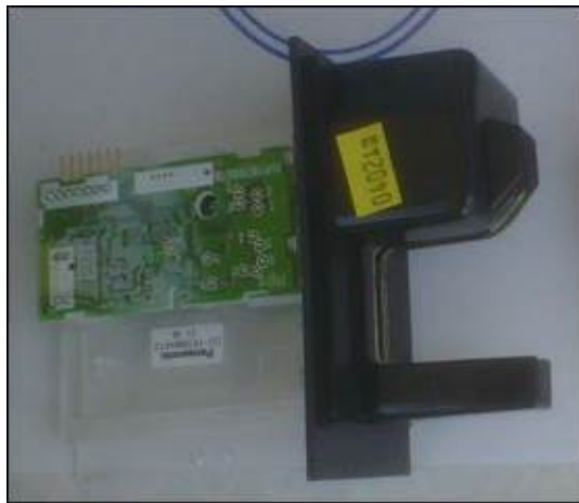
Figure 5.14: A skimming device removed from a gas pump.
