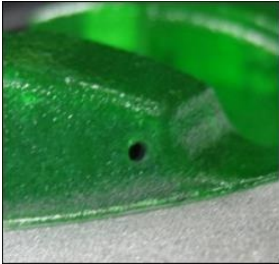
Figure 5.12: A pinhole camera embedded into a card skimmer.
