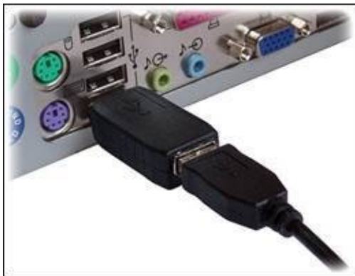
Figure 1.14: A hardware key logger between a computer and keyboard cable.
