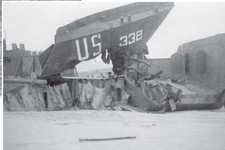
The result of striking a mined obstacle. This is LCT-332. The mine has torn the loading ramp and right front bow off.
