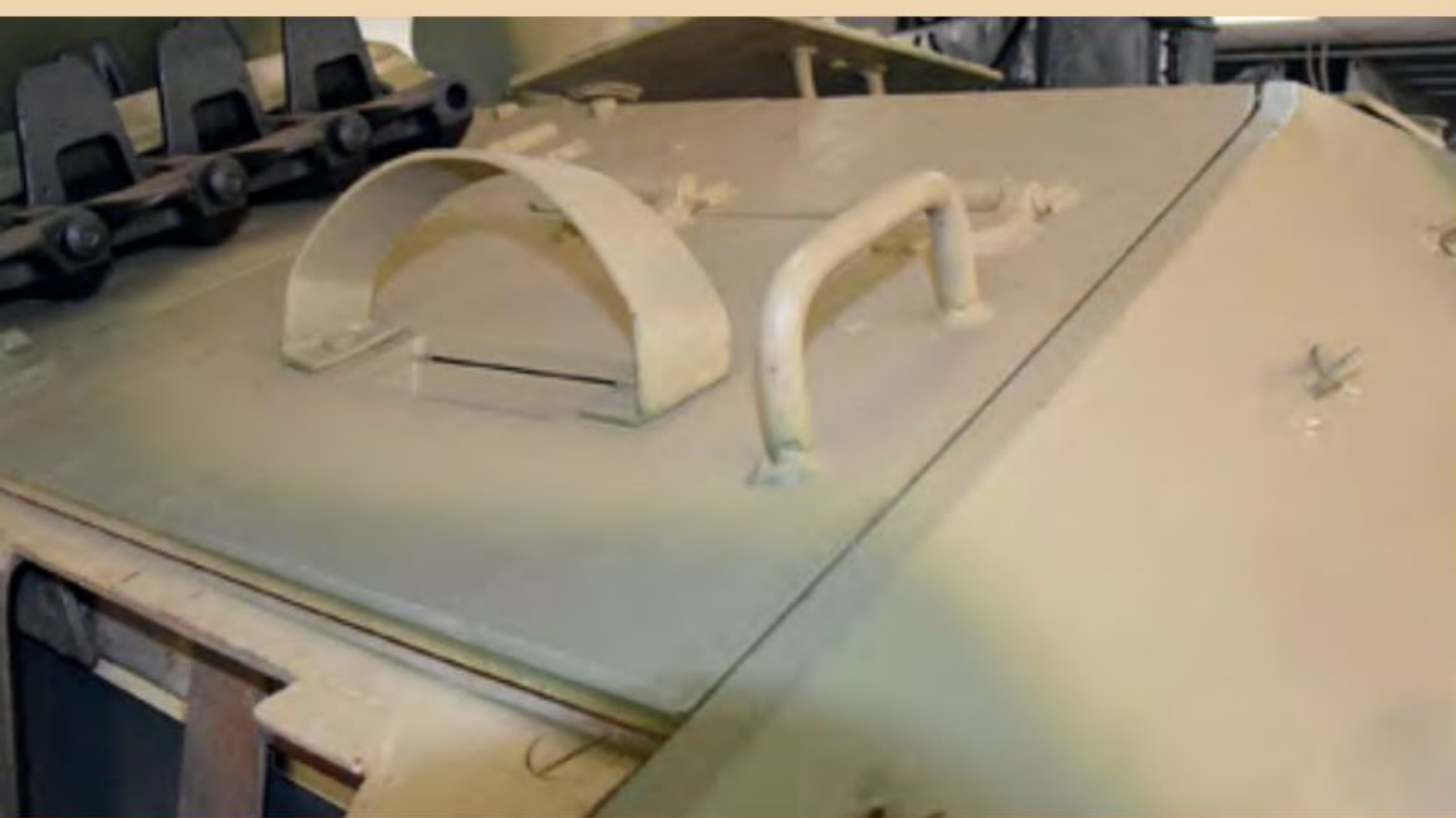
The commander's rear-view periscope (missing) was protected by a curved piece of metal
