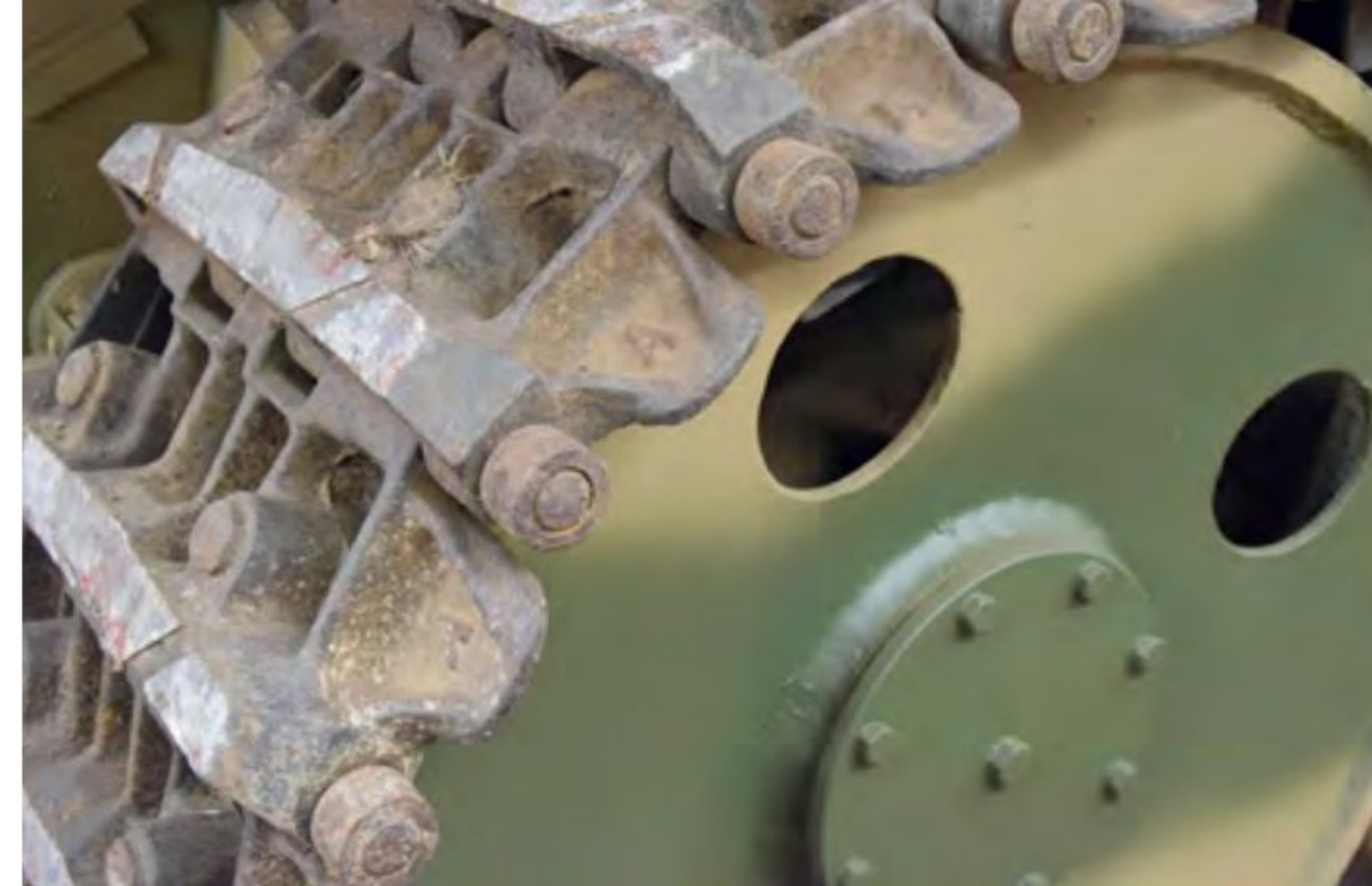
The Jagdpanzer 38 tracks were 35cm wide. The Panzer 38(t) tank tracks were only 29cm wide. Several different styles of rear idler wheels were fitted to the vehicle between 1944 and 1945
