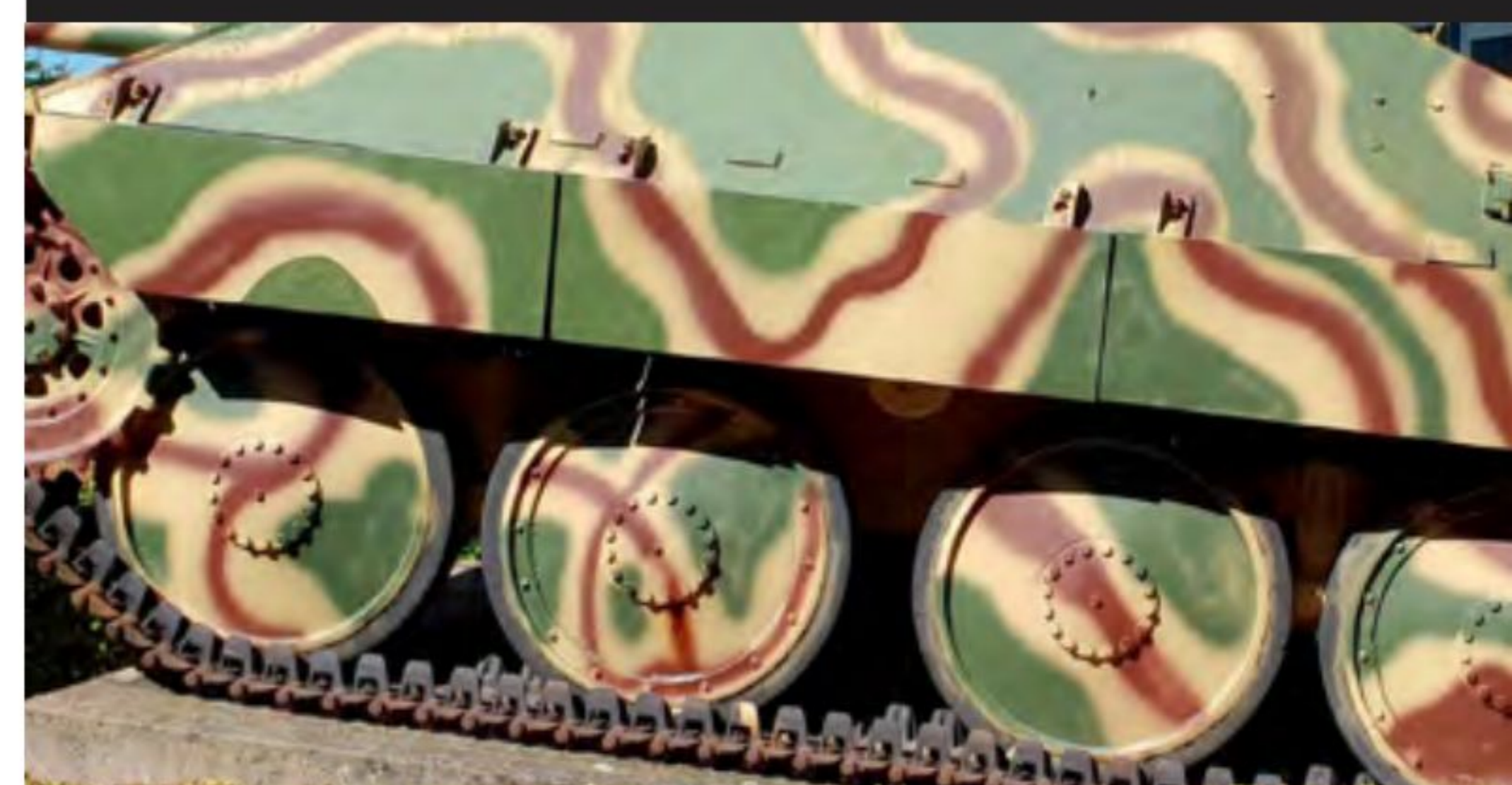
The Schürzen side skirt armour was made from 5mm steel plate. It was designed to protect the side 20mm thick lower hull armour from the Soviet 14.5mm anti-tank rifle
