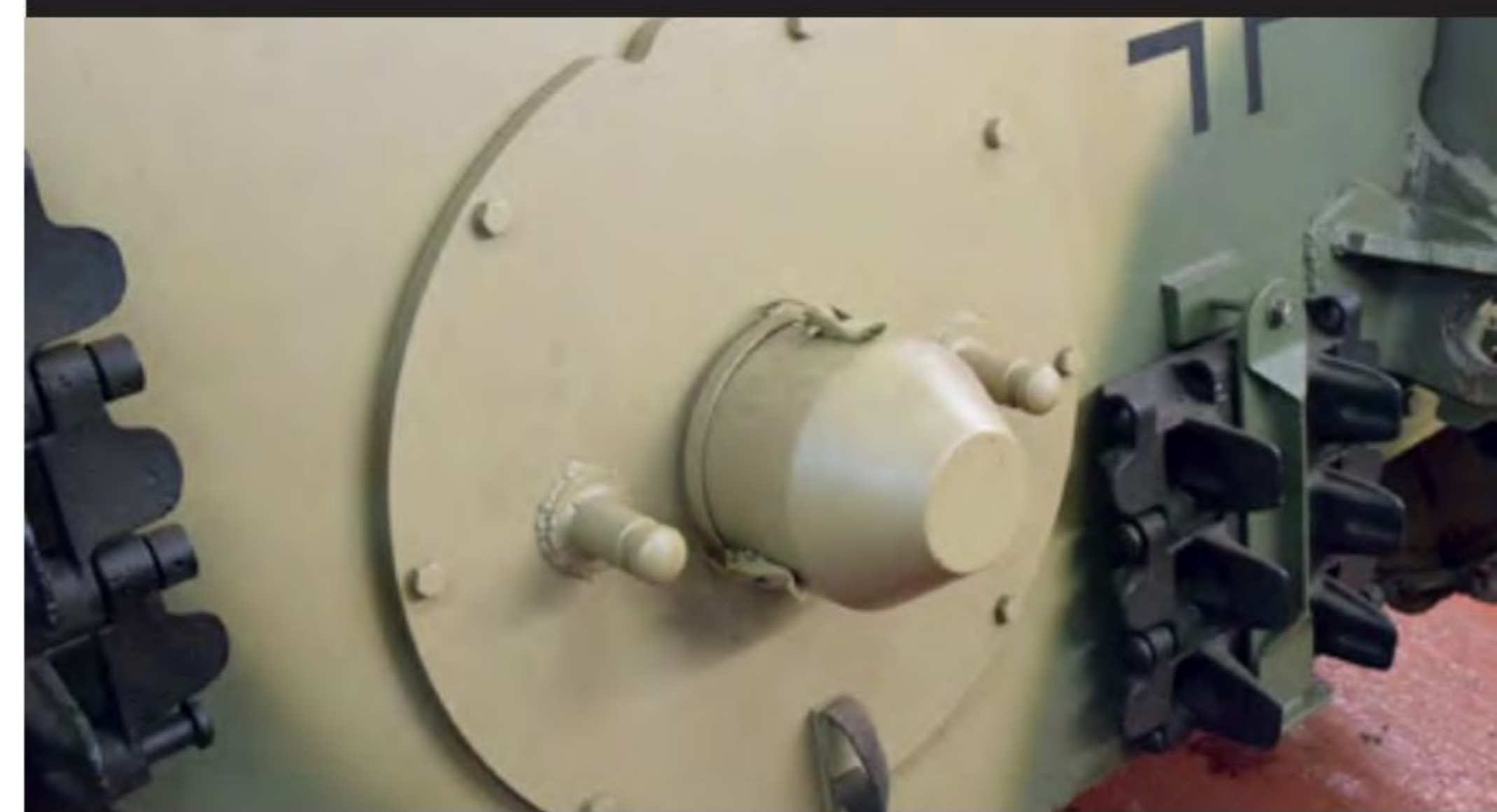
The metal cone in the middle of the bolted circular engine access hatch is a cap that covers the hole for the engine starter hand crank
