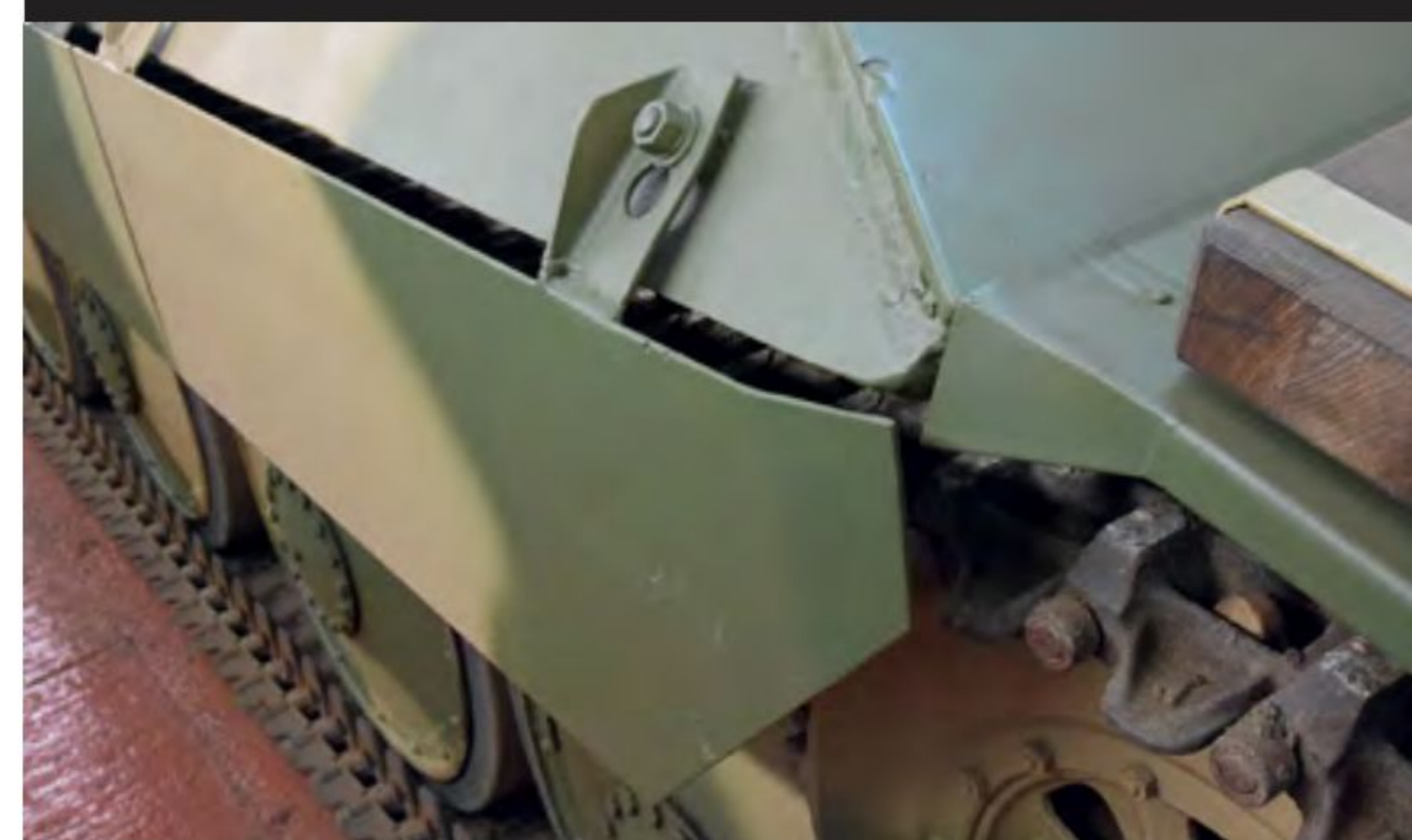
The factory bent the leading edge of the Schürzen side skirt armour to try and prevent it being ripped off by getting caught on branches
