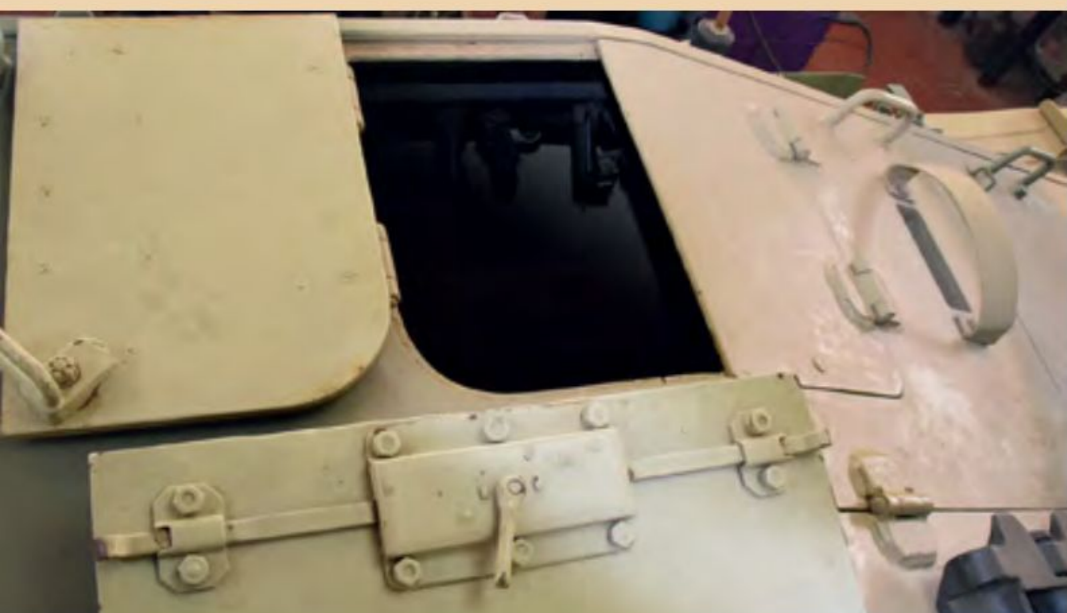
The Jagdpanzer 38 commander did not have a protective armoured cupola. This was his two-door hatch. He had a rearward-looking periscope
