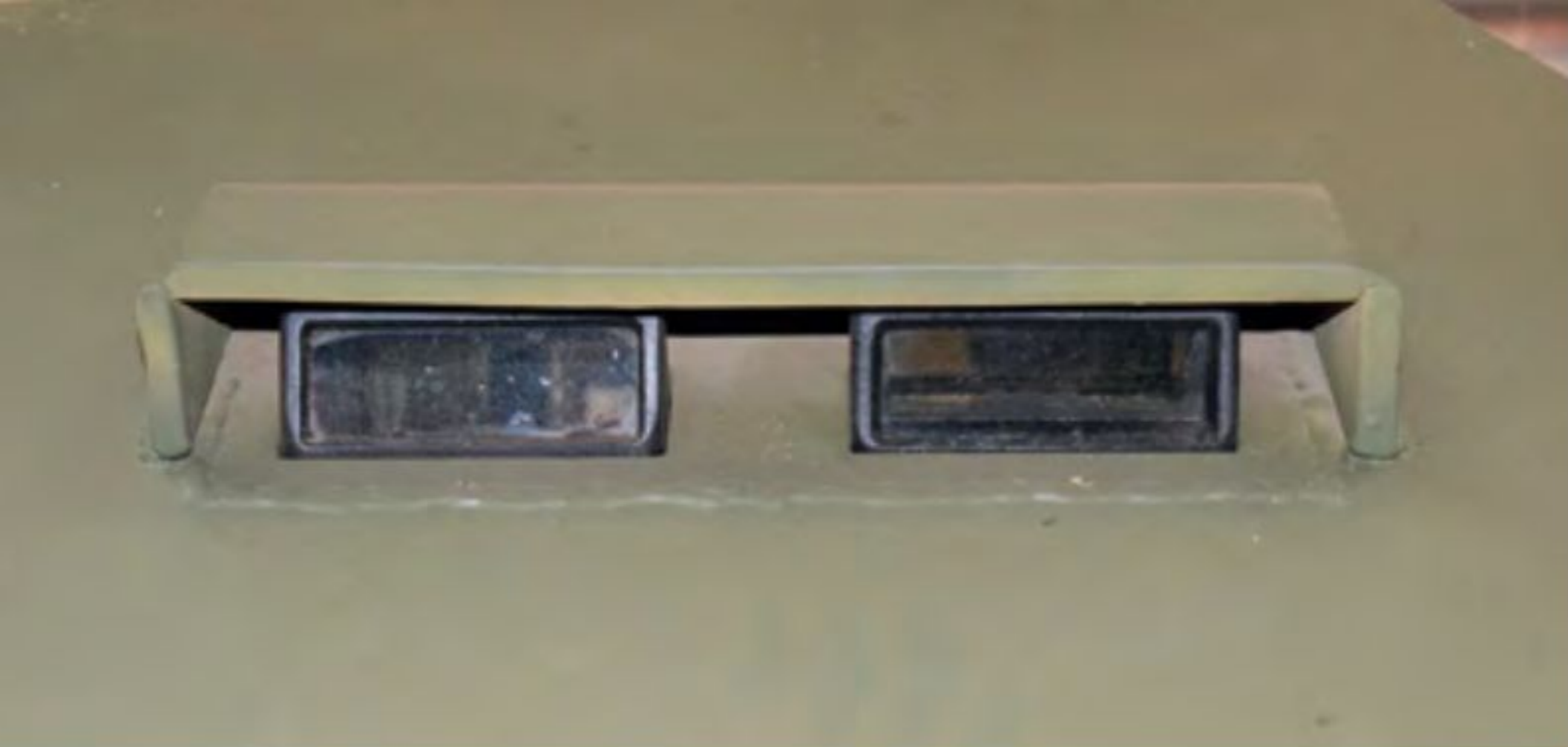
The driver had two forward-looking periscopes. He had no vision to his left or right
