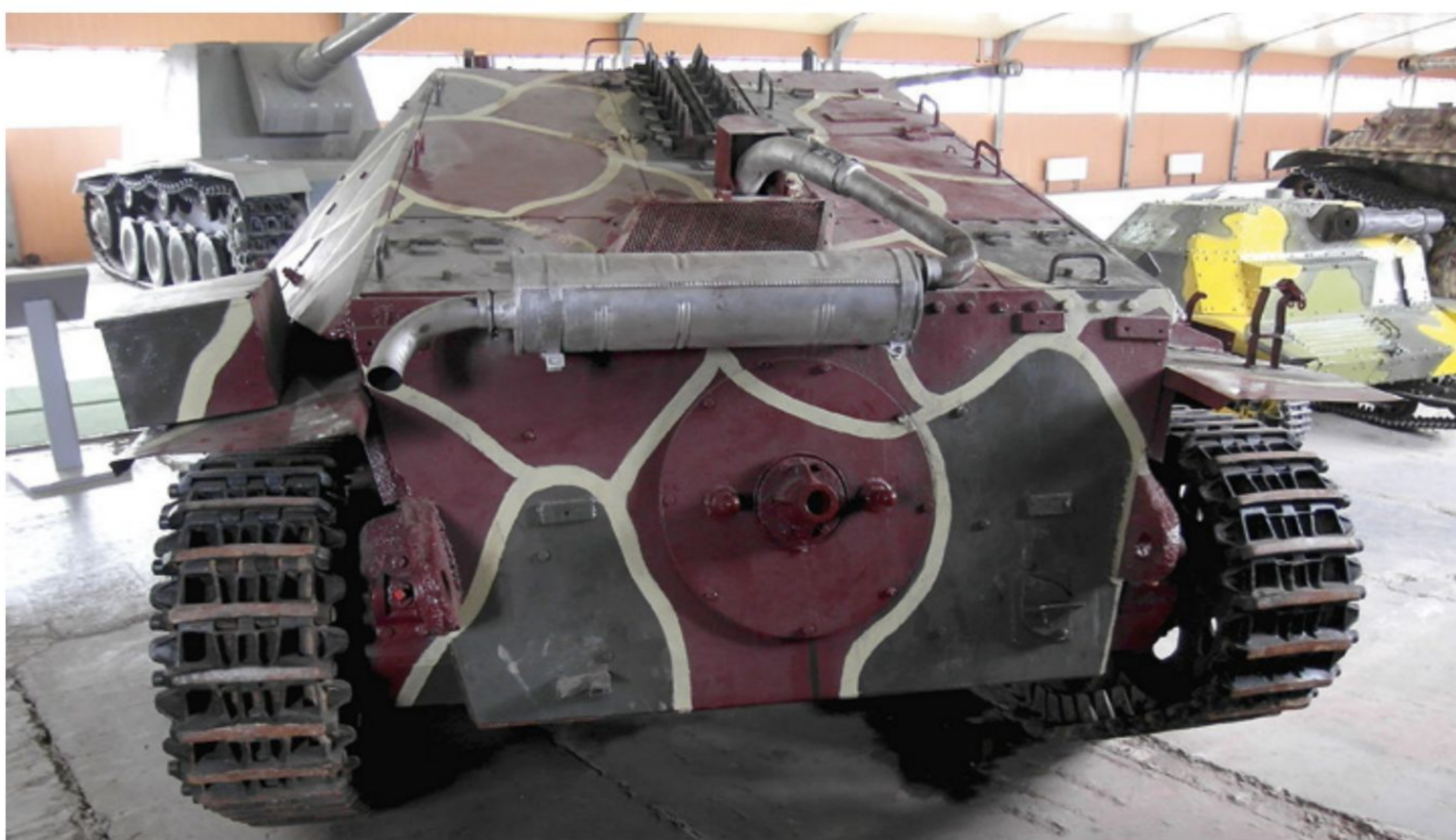
BELOW: The Jagdpanzer 38 on display at the Tank Museum, Kubinka, Russia is fitted with the early version of the exhaust system that had a large horizontal silencer box
