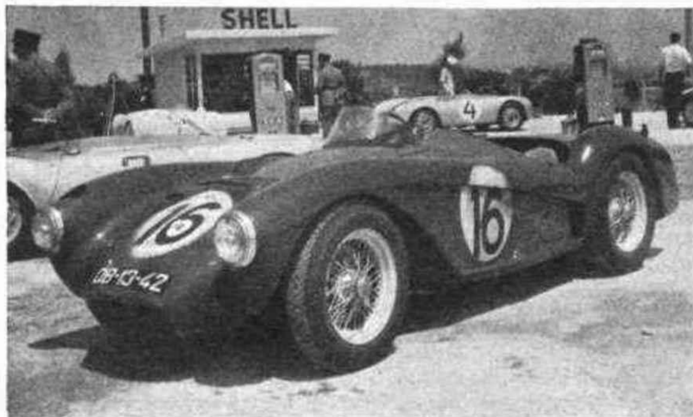
HOME-BUILT. —This attractive-looking "special" was built in Lisbon and utilises an M.G. engine and gearbox in a tubular frame, with Porsche front-end and brakes, A70 Austin rear axle, with Porsche brakes, and a locally-built body.
