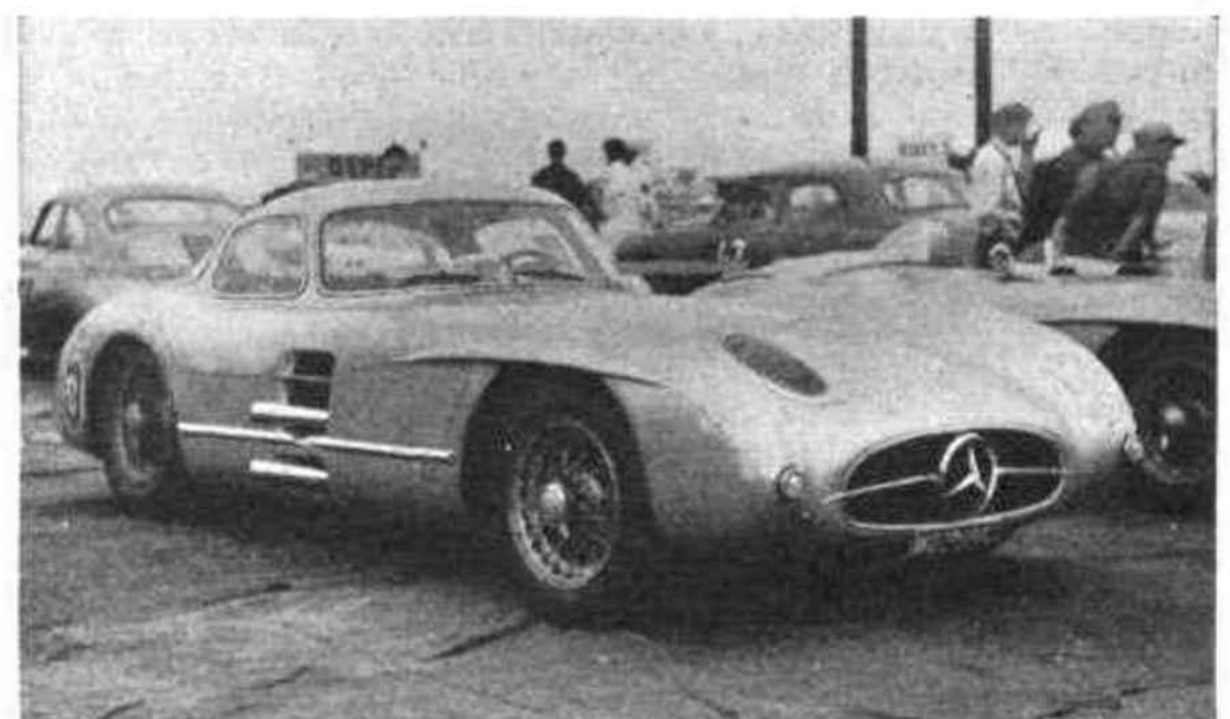
EVOLUTION. —This Mercedes-Benz 300SLR coupé is mechanically identical to the well-known SLR sports/racing cars driven by Fangio and Moss. The coupé body is similar to a 300SL, with "gull-wing" doors and the eight-cylinder engine gives a maximum of over 170 m.p.h.
