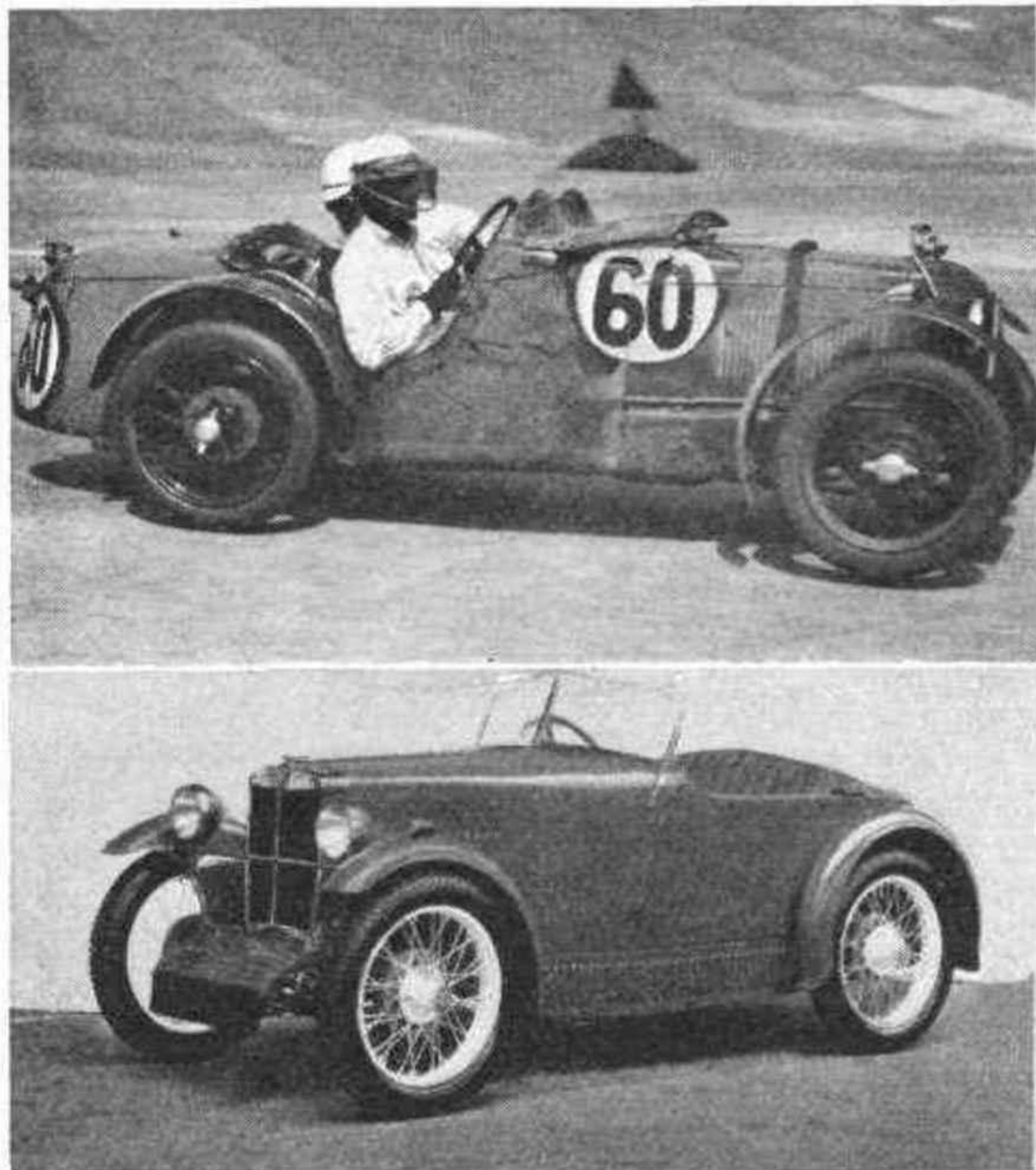
FOR SPORT AND PLEASURE. —Before the war Abingdon raced special versions of the M.G. Midget, which you could also buy, like the 746-c.c. Monlhery C-type driven by the Earl of March and C. S. Staniland in the 1931 J.C.C. "Double Twelve" at Brooklands, in order to popularise the normal 850-c.c. M.G. Midget sports model. The C-type was available ready to race, every nut split-pinned, for £295 and gave 37½ b.h.p. at 6,000 r.p.m., against 20 b.h.p. at 4,000 r.p.m. of the M-type Midget.
