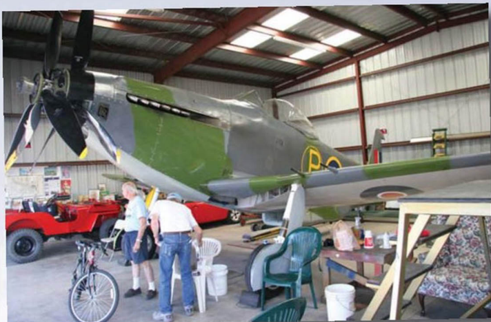
BELOW LEFT and RIGHT: Two views of the replica MB5 that has been built by John Marlin in Reno, Nevada using wings from a North American P-51 Mustang. (Both images courtesy of Bart Hunt)
