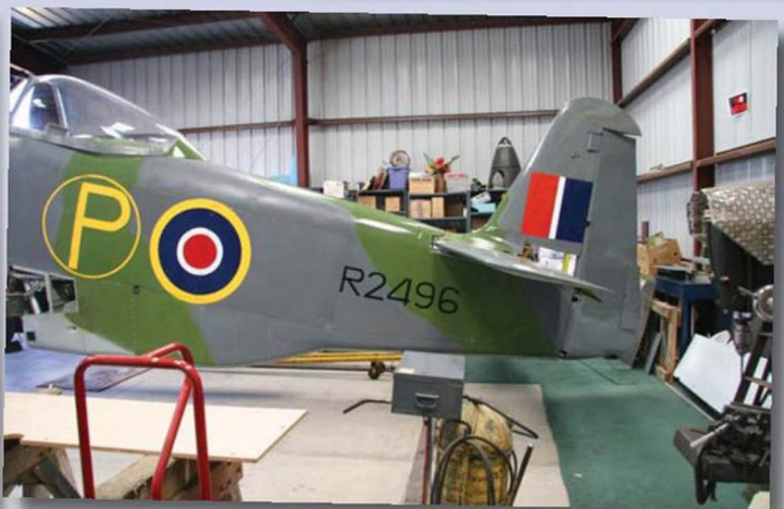
BELOW LEFT and RIGHT: Two views of the replica MB5 that has been built by John Marlin in Reno, Nevada using wings from a North American P-51 Mustang. (Both images courtesy of Bart Hunt)
