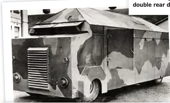
BELOW: What was once an AEC Regent double-decker bus has been converted into an armoured personnel carrier for the London Passenger Transport Board Home Guard. The driver had his own hinged armoured door, with the passengers gaining access through double rear doors.
