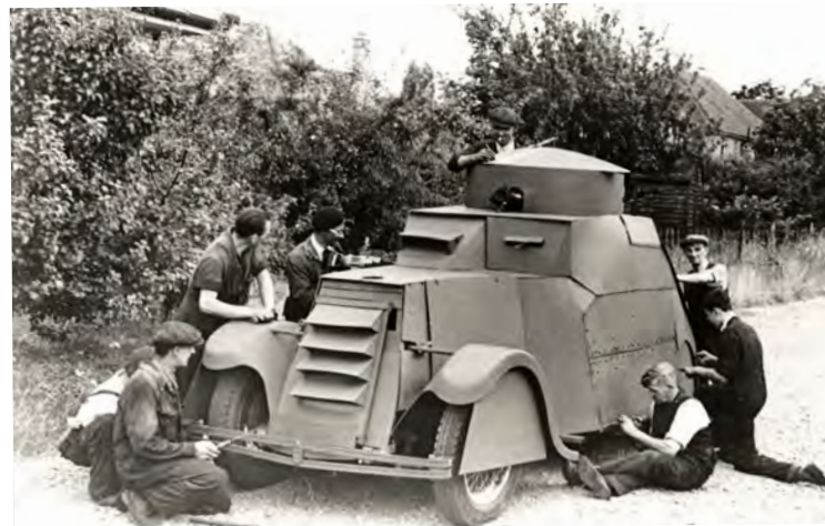
LEFT: A revised design of the Tickler armoured car, with improved driver's visibility, a co-driver's position and the addition of a revolving turret.
