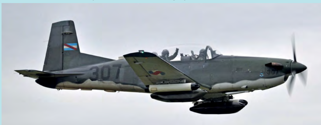
Below: An AT-92 (PC-7) trainer complete with twin MAG machine gun pods and FN Herstal LAU-7H rocket-launchers.
