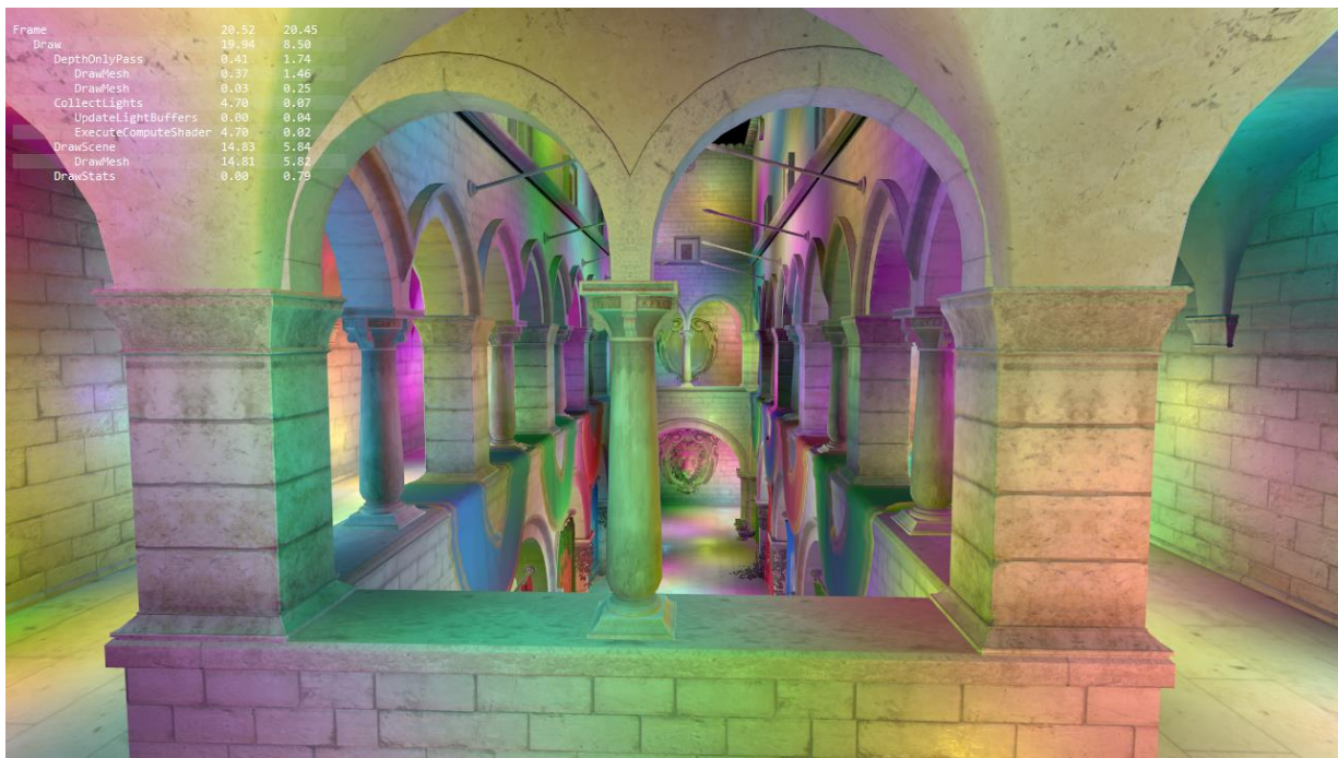
Figure 16 – Final rendered scene at Camera 5 Rendered at 1280x720 resolution, with Hybrid Culling, 8x MSAA, and 1024 lights.
