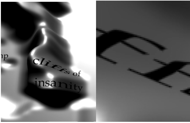
Figure 10: A map using a vector texture for labels, with an enlargement of a distorted region to demonstrate anisotropic antialiasing.
