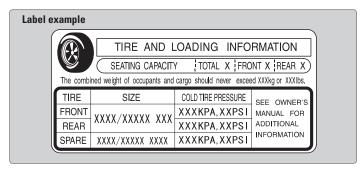
This figure includes the total weight of all occupants, cargo, and accessories, and the tongue load if you are towing a trailer. Below are the steps for determining the correct load limit:
