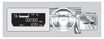
Press the TRIP knob to cycle through the displays shown below.
