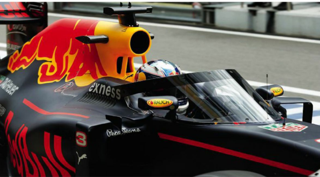
The aeroscreen pioneered by Red Bull is favoured over the halo due to its greater frontal protection
