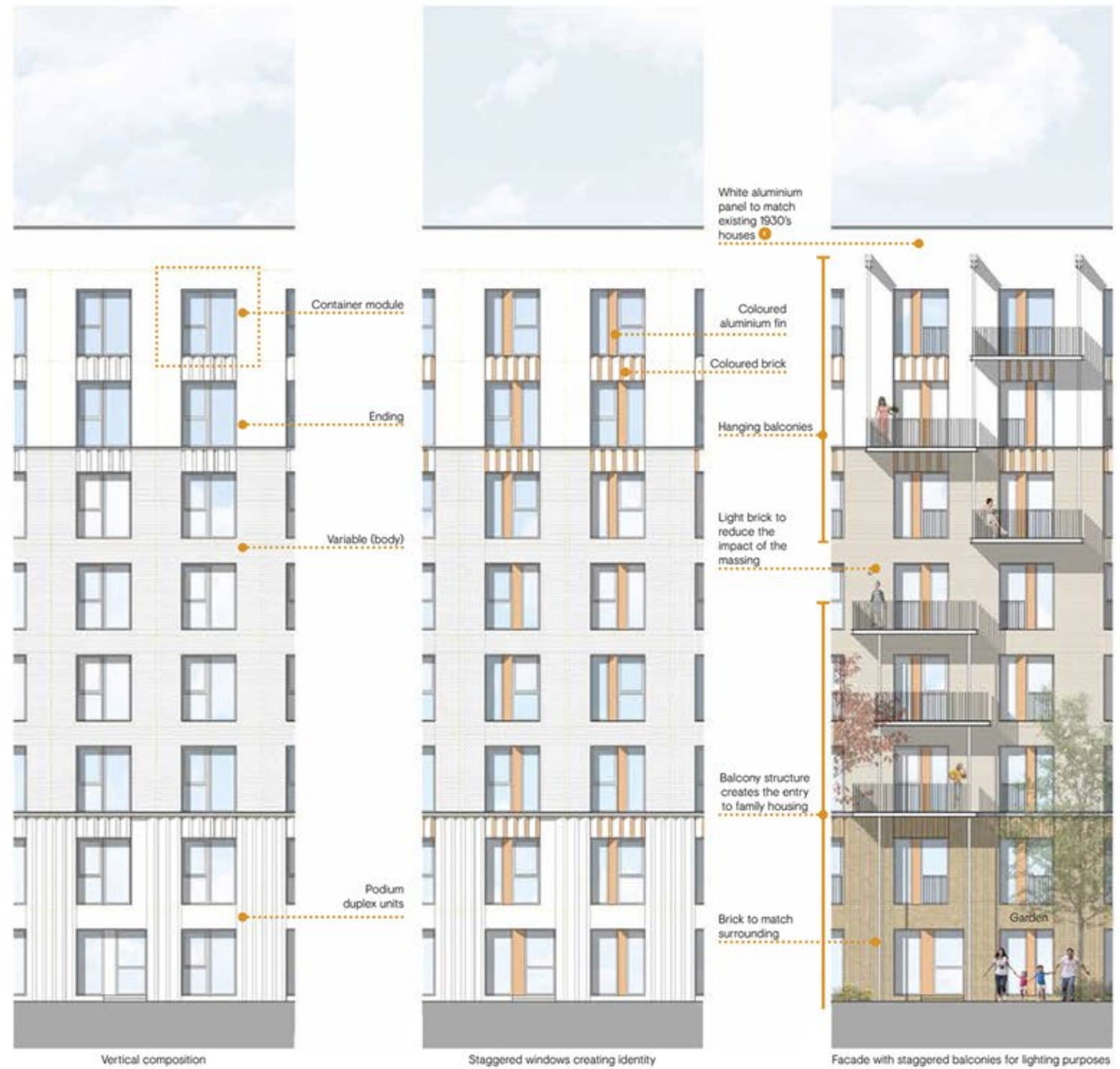
FACADE STUDIES. CIMC sea containers are clad with brick. Within a frame of respect of the urban environment the facade design searches to create identity for the user
