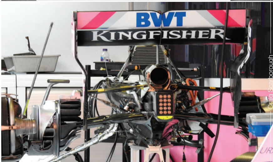
ABOVE & BELOW The power unit, gearbox and hydraulics package are all sourced from Mercedes HPPT. That tie up could be set to get closer still
