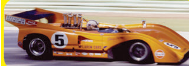
1971 McLaren M8F Can Am car. Ran Kinsler prepared MacKay intake Manifold with Lucas mechanical metering.
